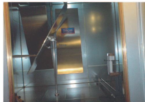
Figure 2. Inside view of RC: showing LPA, bowtie antenna on horizontal slider and stirrers.
