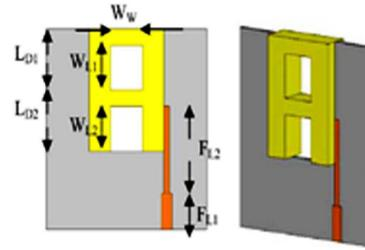
**Figure 20.** A-shaped DRA mounted on a vertical ground plane edge [101].
