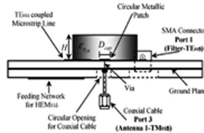
**Figure 22.** Side view of the triple mode DRA [116].
