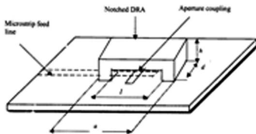
**Figure 1.** Notched rectangular DRA with aperture slot coupling [6].
