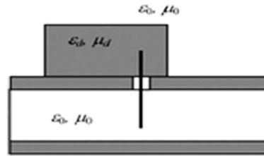
Figure 6. Waveguide-probe-excited circular disk DRA [35].
