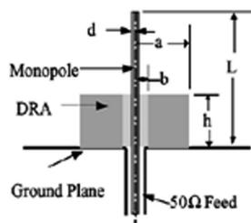
Figure 15. Cross section of the hybrid monopole-DRA [79].
