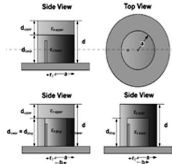
**Figure 10.** Stacked and embedded cylindrical DRA [52].
