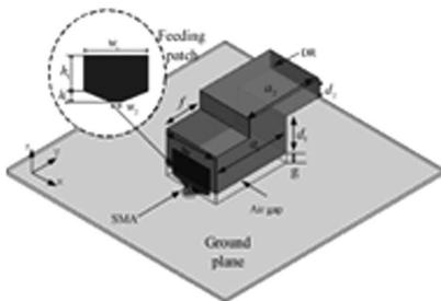
**Figure 17.** Geometry of Z-shaped UWB DRA [96].
