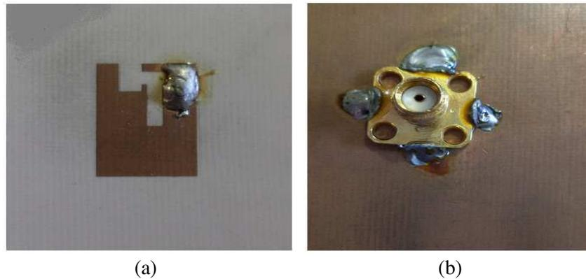
Figure 2. Photograph of fabricated antenna 1 (a) patch, (b) ground plane.
