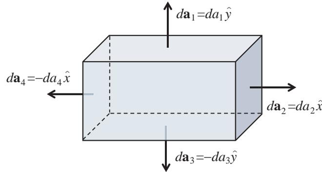
**Figure 3.** Cuboid with its surface elements for four sides shown representing the lower Halbach array in the dual configuration (for clarity the upper array isn't shown).
