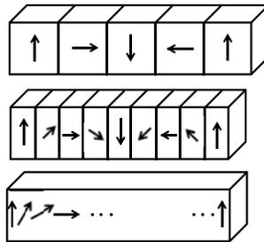
**Figure 1.** Two discrete (with  $m = 5$  and  $m = 9$ , respectively) and one continuous (bottom) Halbach array. The wavelengths of the magnetization are in all the three cases equal to the individual widths of the arrays.
