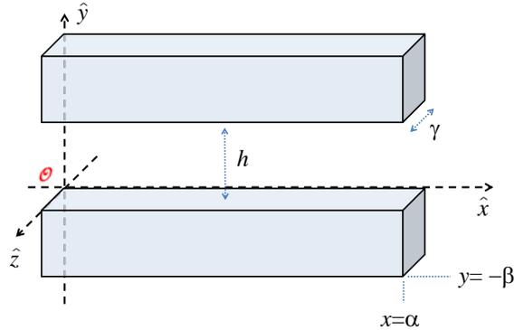
**Figure 2.** Two Halbach arrays with opposing magnetization (e.g., “North-North”) is used in a dual configuration. The two arrays have identical dimensions of  $\alpha$ ,  $\beta$  and  $\gamma$  (i.e., width, height and depth).
