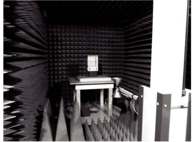
**Figure 10.** Fully automated measurement setup in semi-anechoic chamber.
