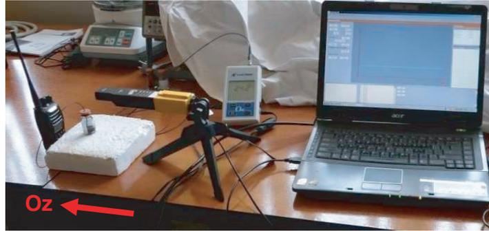
**Figure 1.** Portable transceiver, magnetic liquid sample to simulate magnetite presence in the brain, fluoroptic probe immersed to measure heating for magnetic-dosimetry, RADMAN XT exposimeter to measure incident field strength and TrueTemp3 software on laptop to record temperature increase.
