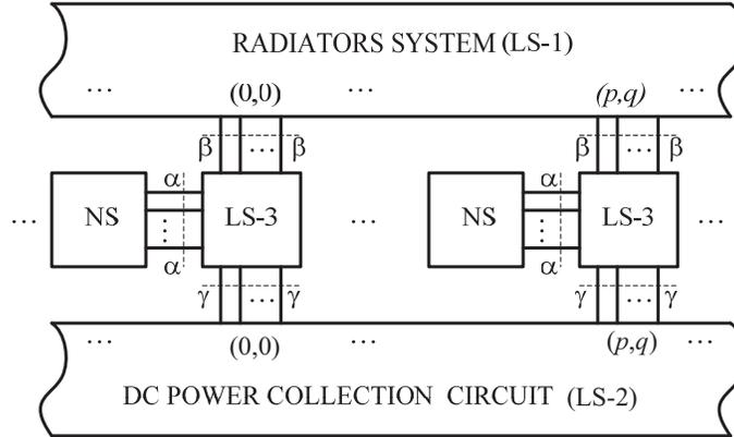
Figure 3. The block-diagram of the rectenna array.
