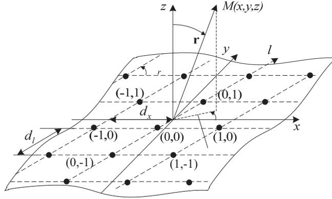
Figure 2. The periodic structure of the rectenna array.
