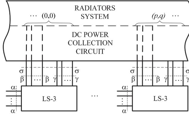
**Figure 5.** The modified linear subcircuit of the rectenna.
