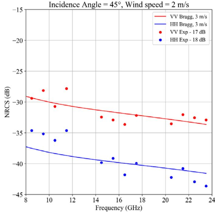
**Figure 9.** Comparison between the measured NRCS in the pool (dots) and the modeled NRCS with the Elfouhaily spectrum for a wind speed at 10 m above the sea surface of 3 m/s (continuous curve) in dB. The experimental conditions are: an incidence angle of  $45^\circ$  and a wind speed of 2 m/s. The *VV* polarization is in red color and the *HH* one in blue color. The mean value of the deviation function  $\Delta$  over the EM frequency range is subtracted from the measured NRCS.
