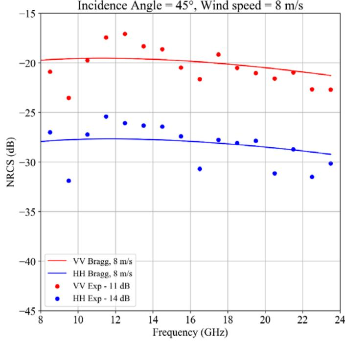
**Figure 11.** Comparison between the measured NRCS in the pool (dots) and the modeled NRCS with the Elfouhaily spectrum for a wind speed at 10 m above the sea surface of 8 m/s (continuous curve) in dB. The experimental conditions are: an incidence angle of  $45^\circ$  and a wind speed of 8 m/s. The VV polarization is in red color and the HH one in blue color. The mean value of the deviation function  $\Delta$  over the EM frequency range is subtracted from the measured NRCS.
