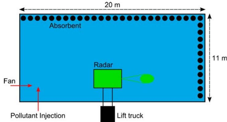
**Figure 1.** Schematic top view of the experimental configuration.
