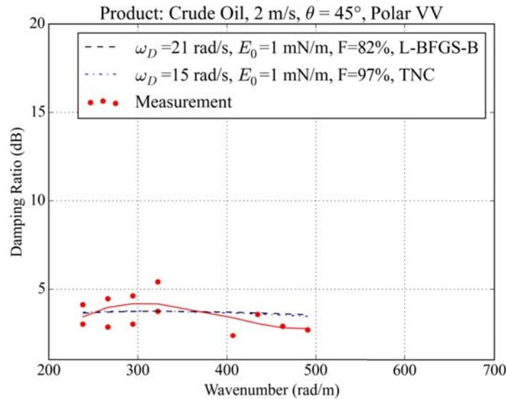
**Figure 14.** Damping ratios calculated for crude oil spill by considering a wind speed of 2 m/s in VV polarization for an incidence angle of  $45^\circ$ . The data points (red dots) are fitted by a third-degree polynomial (red line). The dashed lines are the damping ratios obtained from the minimization process (black dashed line: L-BFGS-B method, blue dotted line: TNC method).
