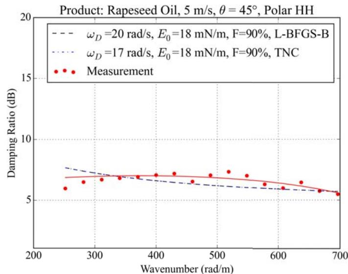
**Figure 15.** Damping ratios calculated for rapeseed oil slick by considering a wind speed of 5 m/s in HH polarization for an incidence angle of  $45^\circ$ . The data points (red dots) are fitted by a third-degree polynomial (red line). The dashed lines are the damping ratios obtained from the minimization process (black dashed line: L-BFGS-B method, blue dotted line: TNC method).
