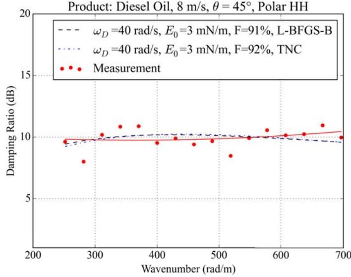
**Figure 16.** Damping ratios calculated for diesel oil spill by considering a wind speed of 8 m/s in  $HH$  polarization for an incidence angle of  $45^\circ$ . The data points (red dots) are fitted by a third-degree polynomial (red line). The dashed lines are the damping ratios obtained from the minimization process (black dashed line: L-BFGS-B method, blue dotted line: TNC method).
