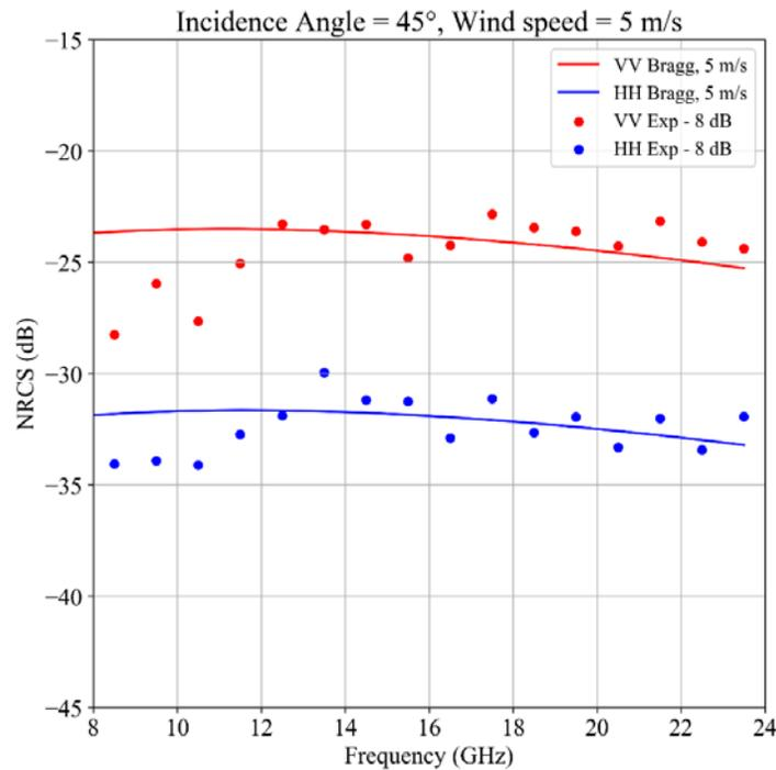
**Figure 10.** Comparison between the measured NRCS in the pool (dots) and the modeled NRCS with the Elfouhaily spectrum for a wind speed at 10 m above the sea surface of 5 m/s (continuous curve) in dB. The experimental conditions are: an incidence angle of 45° and a wind speed of 5 m/s. The VV polarization is in red color and the HH one in blue color. The mean value of the deviation function  $\Delta$  over the EM frequency range is subtracted from the measured NRCS.
