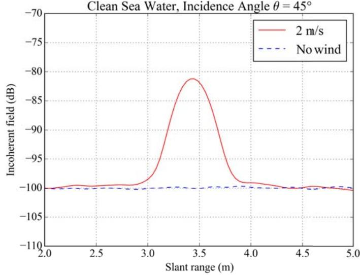
**Figure 7.** Incoherent field of the clean seawater surface with an incidence angle of  $45^\circ$  in  $VV$  polarization at 10.5 GHz. Two configurations are observed: a seawater state with a wind speed of 2 m/s (red line) and a flat seawater surface (blue dashed line).
