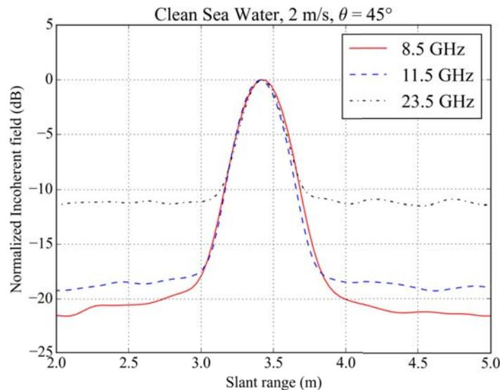
**Figure A1.** Normalized incoherent field of the clean seawater surface with an incidence angle  $45^\circ$  and a wind speed of 2 m/s in  $VV$  polarization. Three EM frequencies are shown: 8.5 GHz (red line), 11.5 GHz (blue dashed line) and 23.5 GHz (black dotted line).
