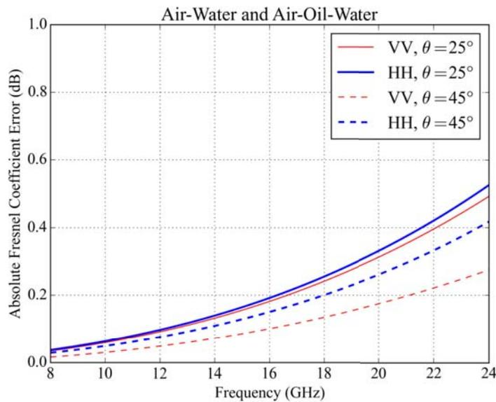
Figure 13. Absolute Fresnel reflection coefficient error with a surface film thickness of 1 mm in  $VV$  (red) and  $HH$  (blue) polarizations. The oil relative permittivity is 2.25 and the oil loss factor is 0.01. The seawater dielectric constant is computed from the Meissner and Wentz model. Two incidence angles are studied:  $25^\circ$  in continuous line and  $45^\circ$  in dashed line.
