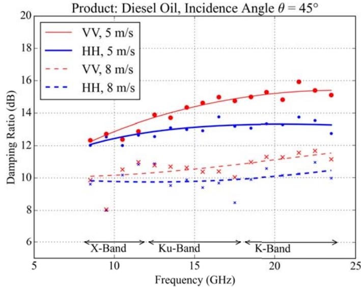
**Figure 8.** Damping ratios from the diesel oil spill acquired at two different wind speeds (5 and 8 m/s) in  $VV$  (red) and  $HH$  (blue) polarizations with an incidence angle of  $45^\circ$ . The lines are third-degree-polynomial fits on the acquired data points (dots and crosses).
