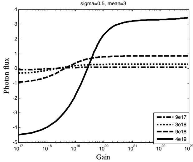
**Figure 3.** Gain vs. photon flux, Er concentration:  $9 \times 10^{17}$ ,  $3 \times 10^{18}$ , and  $4 \times 10^{19} \text{ cm}^{-3}$ ,  $\delta$ : 0.5 nm and mean value: 3 nm.
