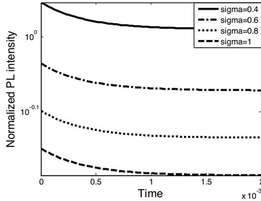
**Figure 10.** Normalized PL intensity vs. Time  $\delta$ : 0.4, 0.6, 0.8 and 1, mean value: 3, Er concentration  $5 \times 10^{20} \text{ cm}^{-3}$ , pump photon flux  $1 \times 10^{19} \text{ cm}^{-2} \text{ sec}^{-1}$ .
