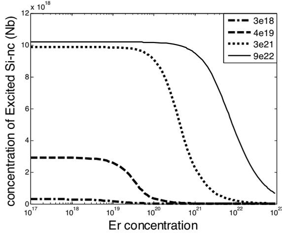
**Figure 5.** Concentration of excited Si-NC vs. Er concentration, pump photon flux:  $3 \times 10^{18}$ ,  $4 \times 10^{19}$ ,  $3 \times 10^{21}$  and  $9 \times 10^{22} \text{ cm}^{-2} \text{ sec}^{-1}$ ,  $\delta$ : 0.5 nm and mean value: 3 nm.
