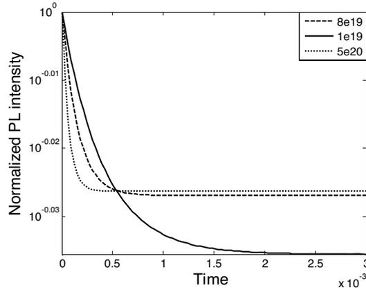
**Figure 8.** Time decay curve of normalized PL intensity pump photon flux:  $1 \times 10^{19}$ ,  $8 \times 10^{19}$  and  $5 \times 10^{20} \text{ cm}^{-2} \text{ sec}^{-1}$ , Er concentration:  $5 \times 10^{20} \text{ cm}^{-3}$ , sigma: 0.5, mean value: 3.
