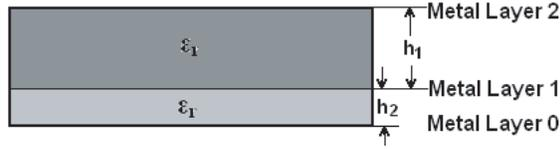
**Figure 2.** Cross section of layers.
