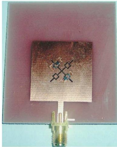
**Figure 2.** Realized patch antenna corresponding to the LHCP mode.
