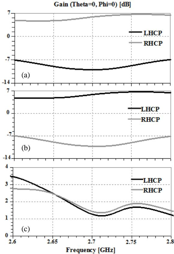
**Figure 5.** LHCP and RHCP Gain calculated by means of full-wave simulations: (a) switches  $R$  on and switches  $L$  off, (b) switches  $L$  on and switches  $R$  off, (c) all switches off.
