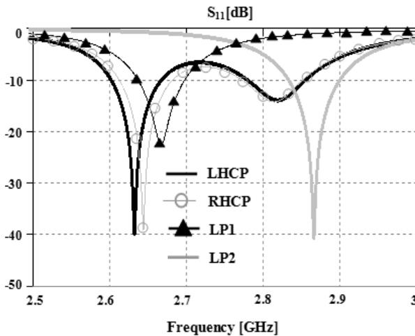
**Figure 3.** Measured return loss of the realized layouts corresponding to the four switch configurations illustrated in Table 1.
