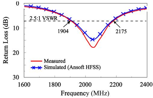
**Figure 2.** Measured and simulated return loss of the proposed antenna with  $d = 5$  mm,  $g = 6$  mm,  $S_2 = 30$  mm,  $S_1 = 46$  mm,  $L = 100$  mm,  $W = 70$  mm; other parameters are given in Fig. 1.
