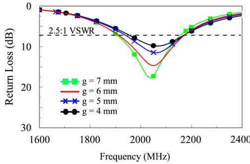
**Figure 6.** Simulated return loss of the proposed antenna with  $g = 7, 6, 5, 4$  mm, respectively;  $d = 5$  mm,  $S_1 = 46$  mm,  $L = 100$  mm,  $W = 70$  mm.
