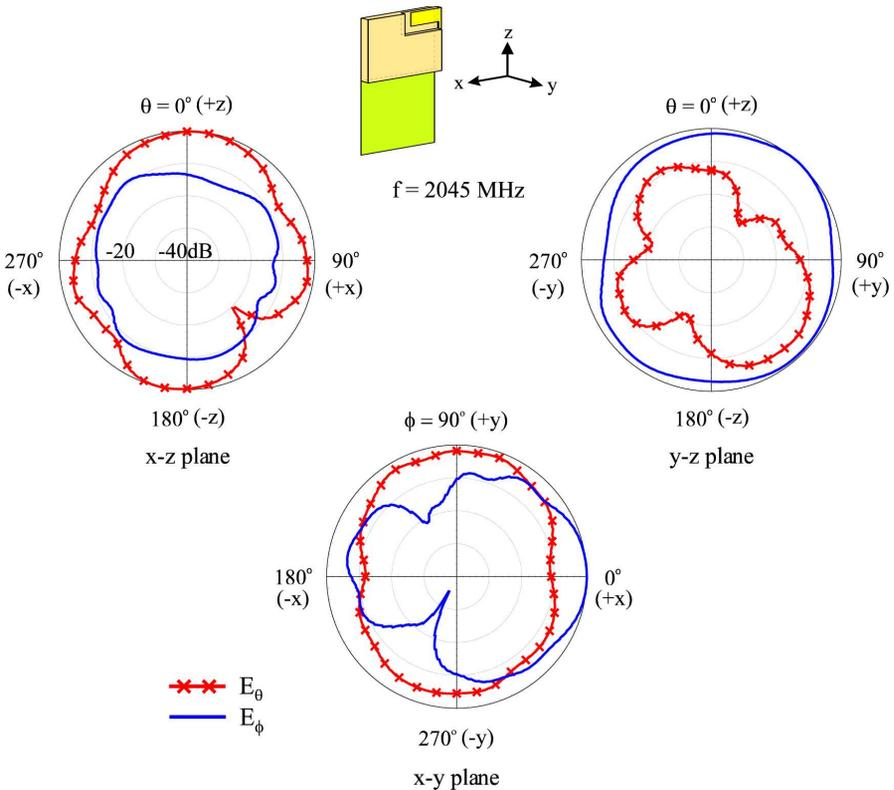
**Figure 3.** Measured radiation patterns at 2045 MHz for the antenna studied in Fig. 2.
