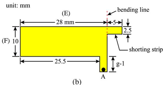
**Figure 1.** (a) Configuration of the internal shorted patch antenna integrated with a shielding metal case for UMTS mobile phone application. (b) Dimensions of the UMTS antenna.
