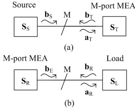
**Figure 1.** Network representation of an  $M$ -port MEA at its (a) Tx and (b) Rx modes of operation.
