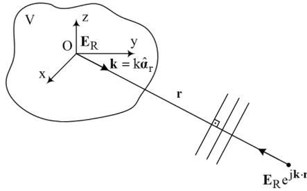
**Figure 4.** The MEA system of Fig. 3 excited by an incident uniform plane wave.
