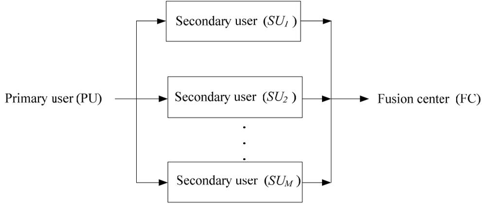
**Figure 1.** Frame structure of cooperative spectrum sensing.
