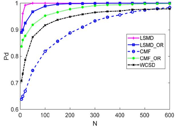
**Figure 3.** The  $P_d$  versus different number of samples of the LSMD, LSMD\_OR CMF, CMF\_OR and WCSD algorithms, where  $P_f = 0.1$ ,  $\text{GSNR} = 2$  dB,  $\alpha = 1.5$ ,  $M = 5$  and  $p_b = 0.2$ .
