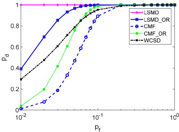
**Figure 2.** ROC curves for a PU with BPSK modulated signal for the LSMD, LSMD\_OR CMF, CMF\_OR and WCSD algorithms, where  $N = 200$ ,  $\text{GSNR} = 2$  dB,  $\alpha = 1.5$ ,  $M = 5$  and  $p_b = 0.2$ .
