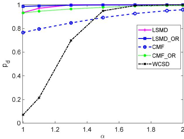
**Figure 6.**  $P_d$  versus different  $\alpha$  of the LSMD, LSMD\_OR CMF, CMF\_OR, and WCSD algorithms, where  $P_f = 0.1$ , GSNR = 2 dB,  $p_b = 0.2$ ,  $M = 5$  and  $N = 200$ .
