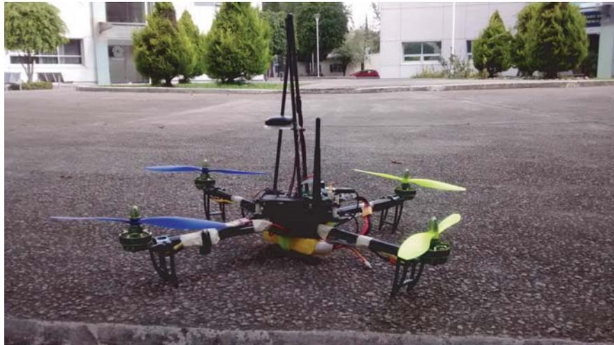
**Figure 2.** Drone with a 2.4 GHz radio onboard.
