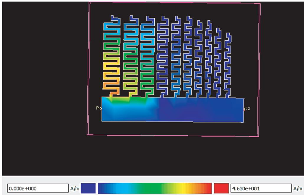
Figure 12. Surface current distribution at 2.1 GHz.
