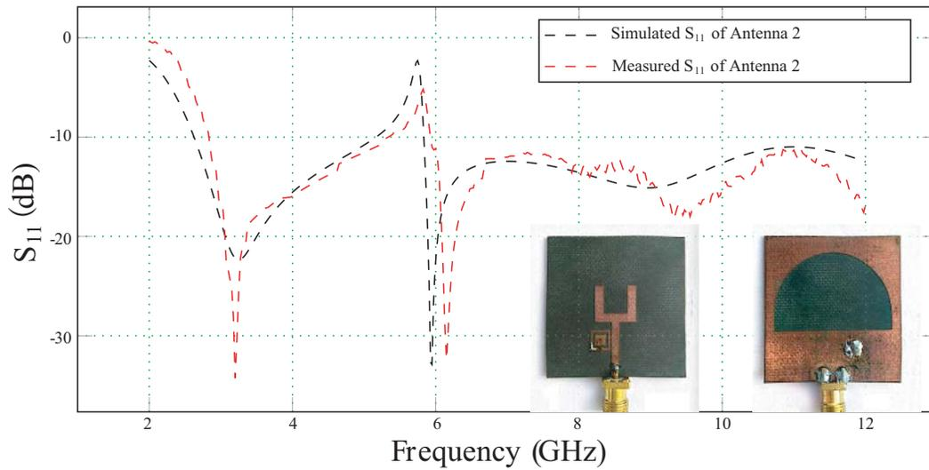
**Figure 9.** Simulated and measured return loss of Antenna 2 with top and bottom view of fabricated prototype.
