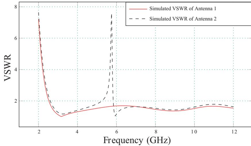
**Figure 5.** Simulated VSWR of Antenna 1 and Antenna 2.
