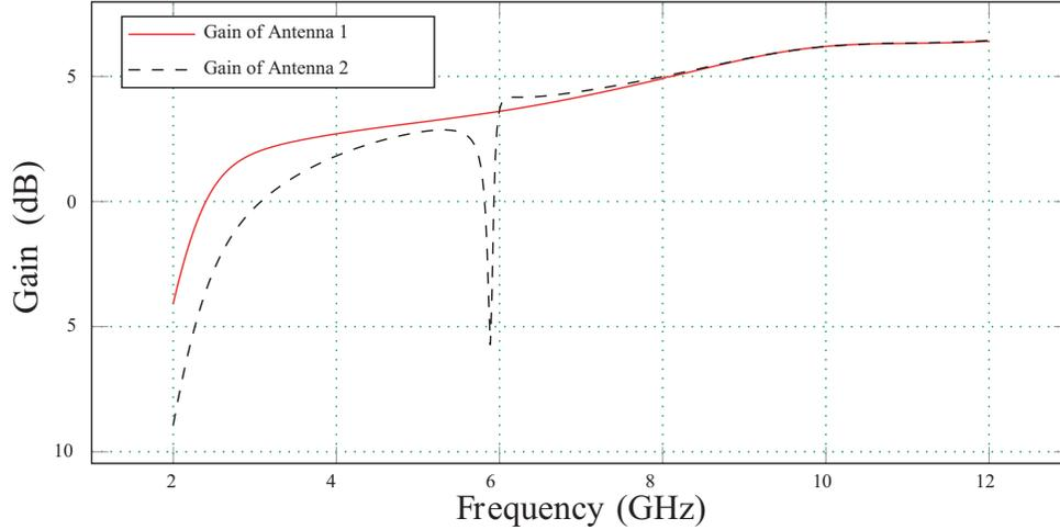
**Figure 7.** Simulated realized gain of Antenna 1 and Antenna 2.
