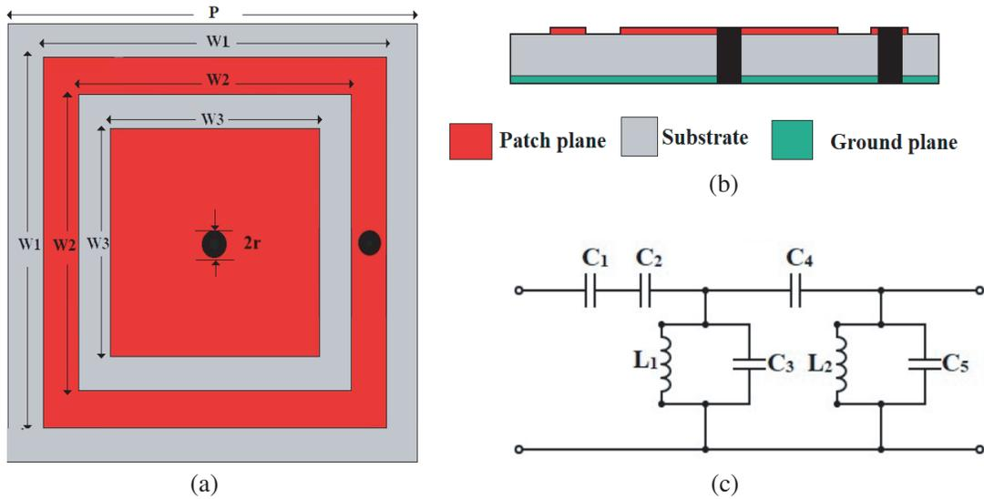
Figure 1. Unit cell of TVS EBG. (a) Top view. (b) Side view. (c) Equivalent circuit diagram.
