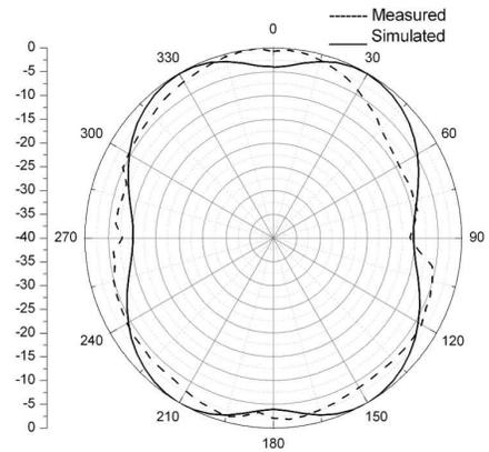
**Figure 16.** *H*-plane radiation pattern at 3.5 GHz.
