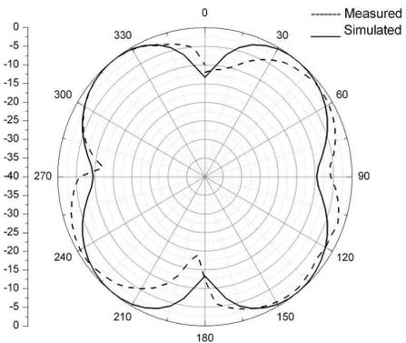
**Figure 14.** *H*-plane radiation pattern at 2.4 GHz.
