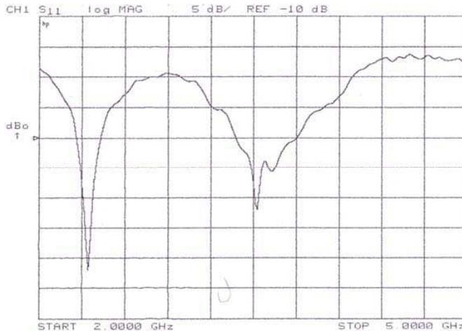
**Figure 4.** The measured return loss of the antenna.
