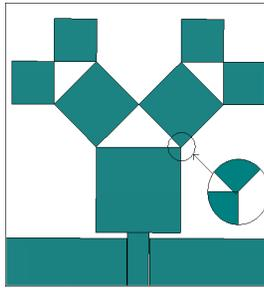
**Figure 2.** Simulated antenna design using CPW feeding.
