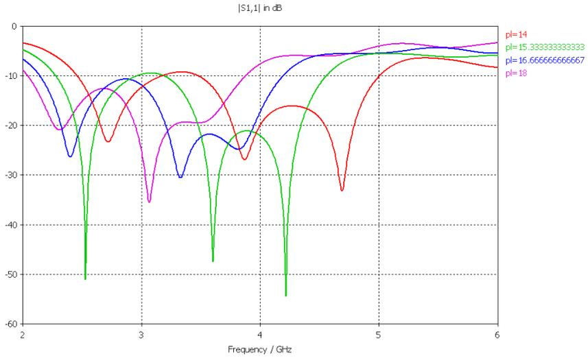
Figure 5. Effect of varying patch length ( $pl$ ).
