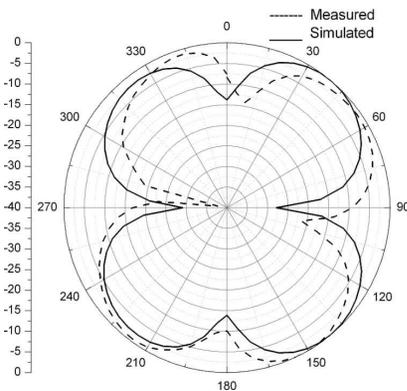
**Figure 13.** *E*-plane radiation pattern at 2.4 GHz.
