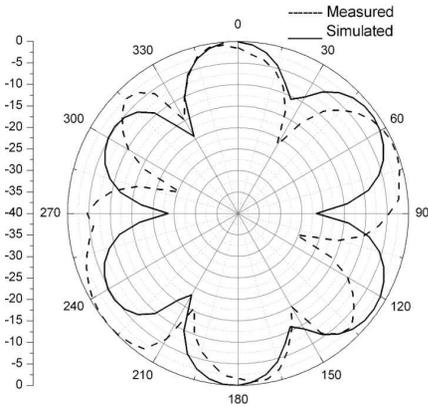
**Figure 15.** *E*-plane radiation pattern at 3.5 GHz.
