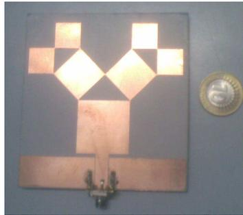
**Figure 12.** Fabricated antenna using Netlec NH9338 as substrate.
