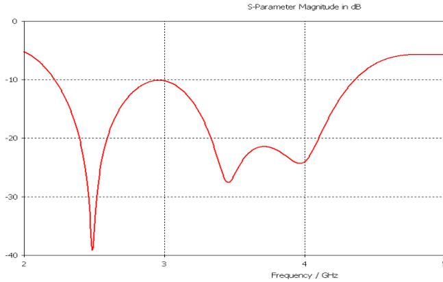
**Figure 3.** The simulated return loss of the antenna.
