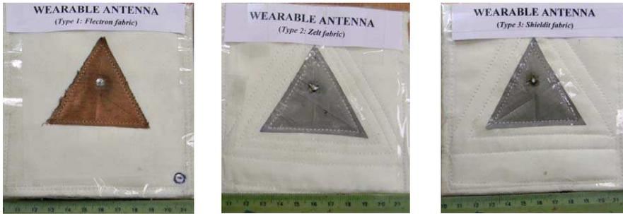
**Figure 2.** Photographs of electro-textile based WiBro antennas developed.
