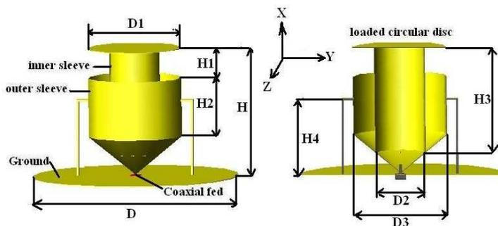
**Figure 1.** Geometry of the proposed antenna.
