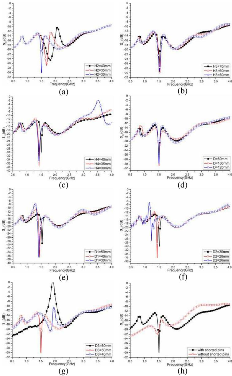
**Figure 2.** Return loss vs. frequency with various parameters. (a)  $H_2$ , (b)  $H_3$ , (c)  $H_4$ , (d)  $D$ , (e)  $D_1$ , (f)  $D_2$ , (g)  $D_3$ , (h) shorted pins.
