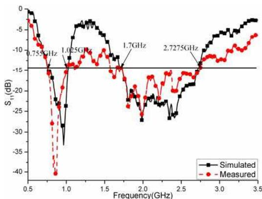
**Figure 4.** Return loss of the proposed antenna.
