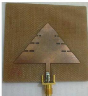
**Figure 7.** Cedar prototype for Case 3 described in Table 1.
