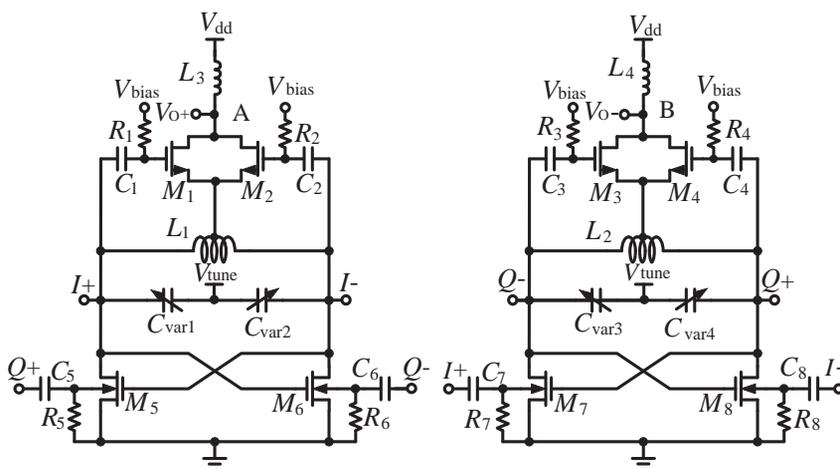
Figure 2. Proposed quadrature VCO using the body injection locked technique.
