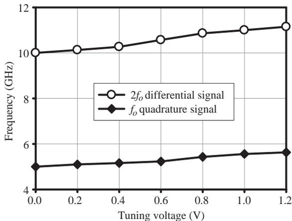
**Figure 6.** Measured tuning range of the VCO and QVCO.  $V_{dd} = 0.9 \text{ V}$ .  $V_{bias} = 1.03 \text{ V}$ .
