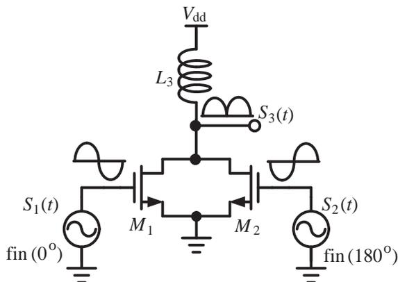
Figure 1. Schematic of a frequency doubler.
