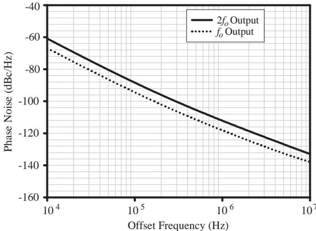
**Figure 4.** Simulated phase noises at the output voltages of  $M_5$  and  $M_1$ .  $V_{dd} = 1\text{ V}$ ,  $V_{bias} = 1.2\text{ V}$ ,  $V_{tune} = 0\text{ V}$ .
