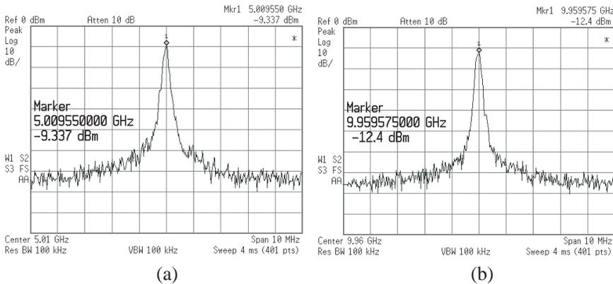
**Figure 7.** Measured spectra of the (a) differential VCO at 9.99 GHz, and (b) quadrature VCO.  $V_{dd} = 0.9$  V, and  $V_{tune} = 0.0$  V.
