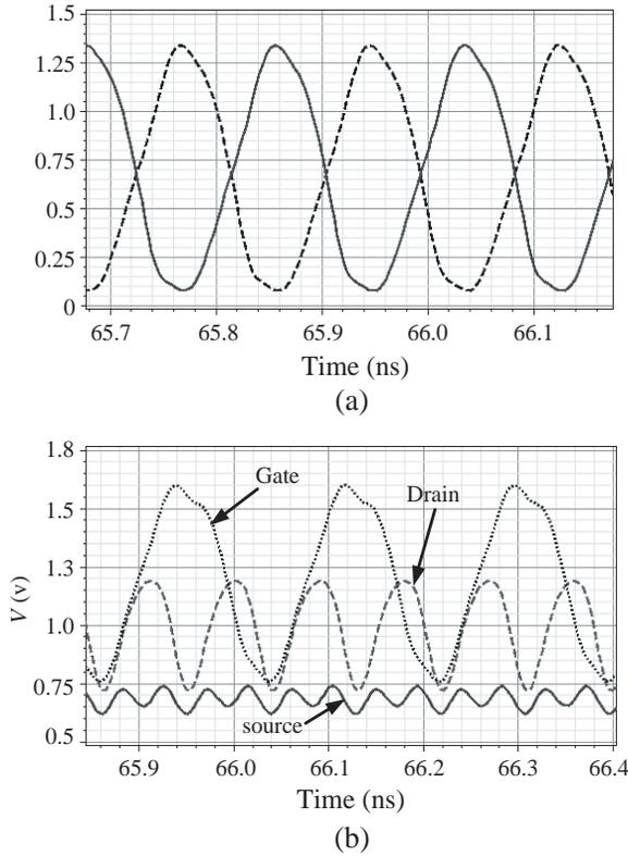
**Figure 3.** (a) Simulated output voltage of  $M_5$  and  $M_6$ . (b) Simulated drain, source and gate voltages of  $M_1$ .  $V_{dd} = 1$  V,  $V_{bias} = 1.2$  V.
