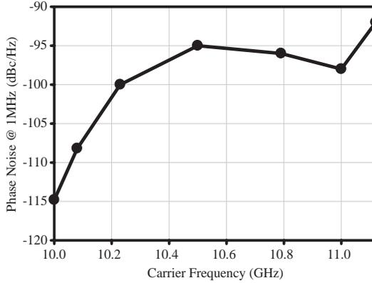
**Figure 9.** Measured phase noise of the differential VCO at 1 MHz offset frequency.  $V_{dd} = 0.9$  V, and  $V_{tune} = 0.0 \sim 1.2$  V.
