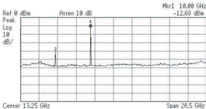
**Figure 8.** Measured full-span spectrum of the differential VCO.  $V_{dd} = 0.9$  V, and  $V_{tune} = 0.0$  V.
