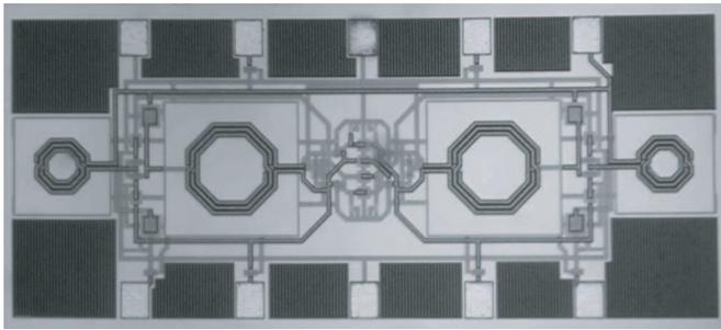
**Figure 5.** Chip photograph of the proposed push-push differential VCO.
