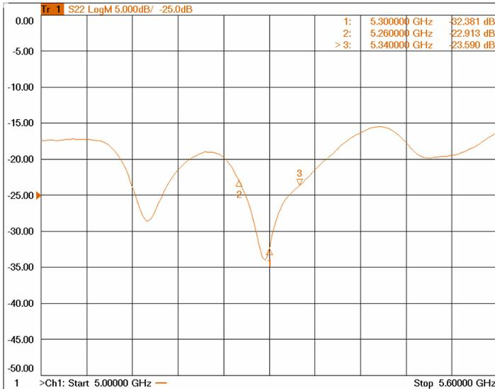
Figure 12. Reflection coefficient of the complete antenna.
