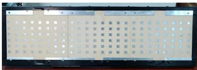
**Figure 9.** Complete antenna with supporting structure.
