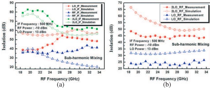
**Figure 6.** Measured and simulated 2LO-to-IF, LO-to-IF, RF-to-IF, 2LO-to-RF, and LO-to-RF isolation levels as functions of the RF.
