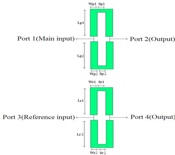
**Figure 6.** Dimensions of the configuration of the proposed double two-section Schiffman phase shifter.
