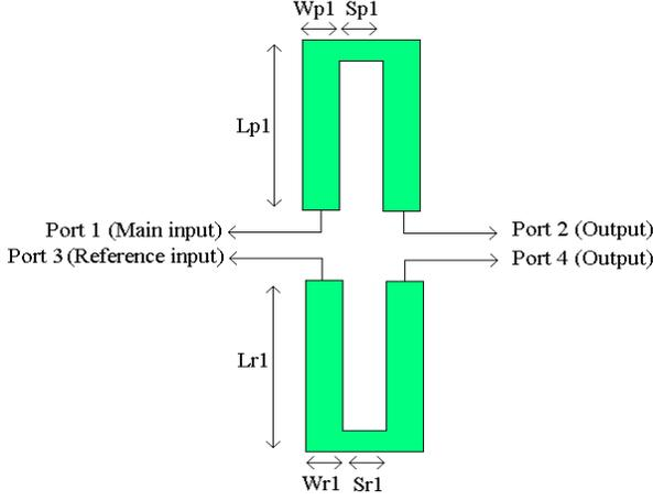
**Figure 2.** Dimensions of the configuration of the proposed single section Schiffman phase shifter.
