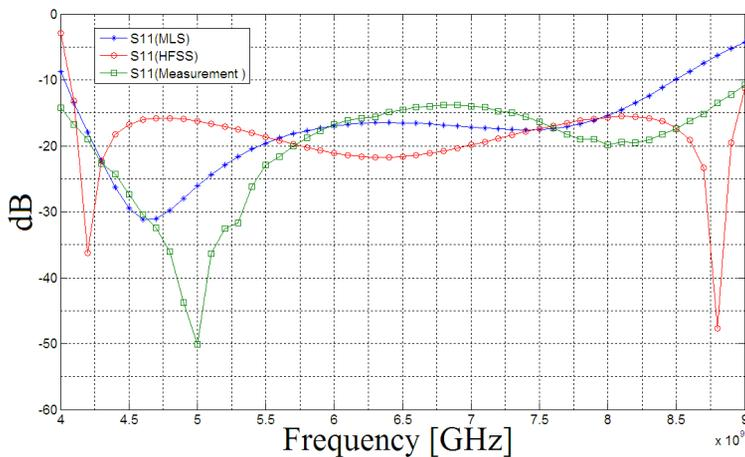
Figure 15. Scattering parameter  $S_{11}$  of example 3.
