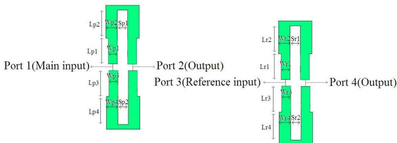
**Figure 12.** Dimensions of the configuration of the proposed double four-section Schiffman phase shifter.
