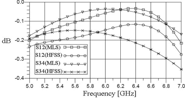
**Figure 5.** Scattering parameters  $S_{12}$  and  $S_{34}$  of example 1.
