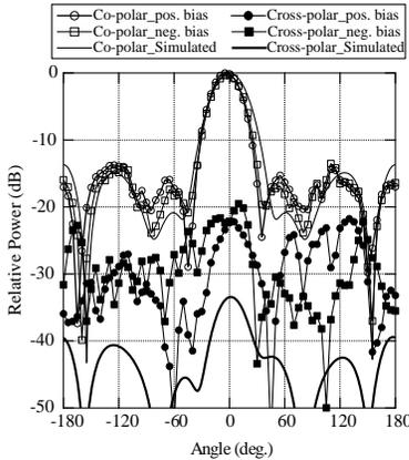
**Figure 7.** The radiation pattern of the array antenna for  $E$ -plane at 3.95 GHz.
