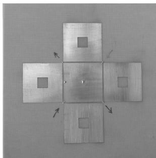
Figure 4. Photograph of the fabricated array antenna.
