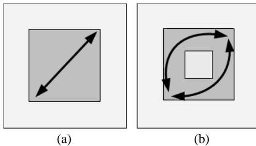
**Figure 3.** The current path of patch containing slot. (a) Without slot. (b) With slot.
