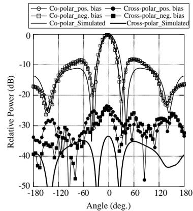
**Figure 8.** The radiation pattern of the array antenna for  $H$ -plane at 3.95 GHz.
