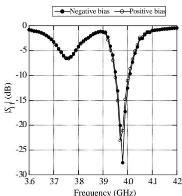
Figure 5. The measured  $|S_{11}|$  characteristics of the array antenna.
