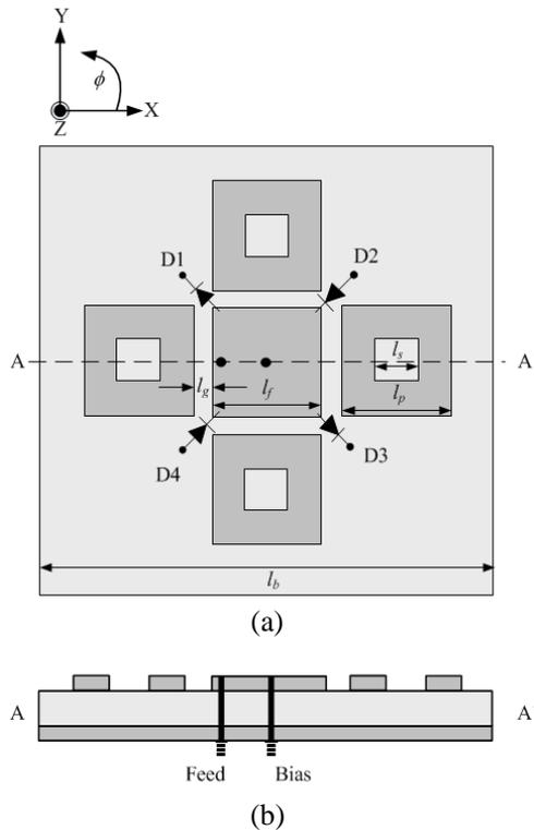
**Figure 1.** Structure of the proposed array antenna. (a) Top view. (b) Cross-section View.
