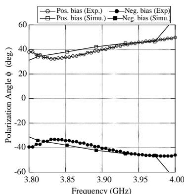
Figure 6. Polarization angle  $\phi$  of the array antenna.
