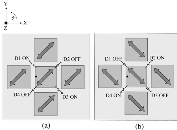
**Figure 2.** Basic behavior of the orthogonal linear polarizations. (a) Positive bias. (b) Negative bias.
