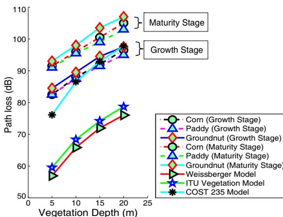
**Figure 4.** Measured and predicted path loss in agricultural fields using RF equipments.
