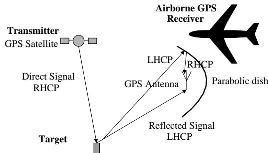
**Figure 1.** Parabolic reflector used to provide gain and change signal polarization.
