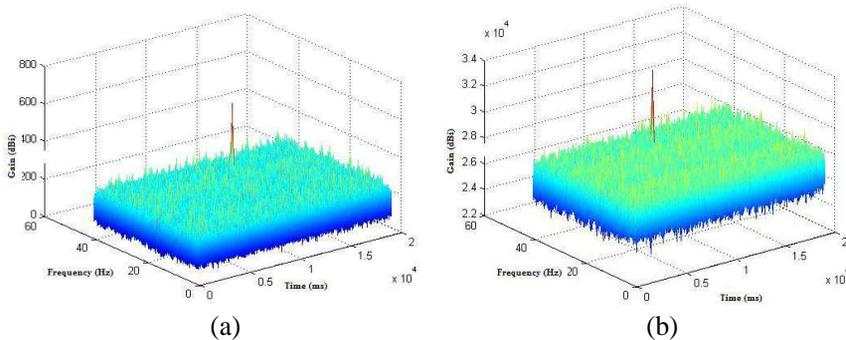
**Figure 4.** Comparison of acquisition plot for (a) Trimble Bullet III antenna (acquisition time of 5 ms) and (b) passive custom made RHCP antenna (acquisition time of 300 ms).
