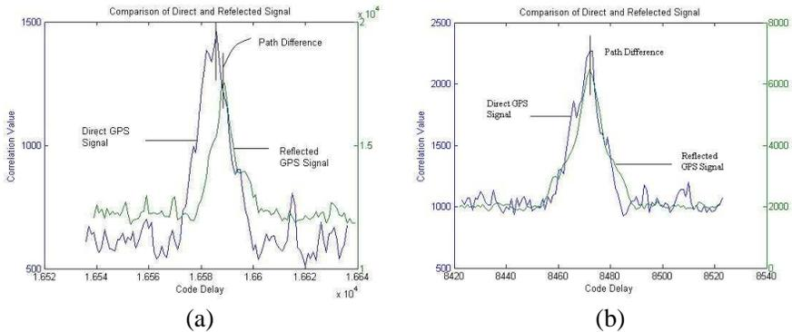
**Figure 8.** Comparison of direct and reflected GPS signals for (a) 50 m, (b) 4 m (round trip distances).
