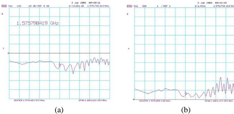
**Figure 3.** VNA plot for the LHCP antenna, showing  $S_{11}$  and VSWR.
