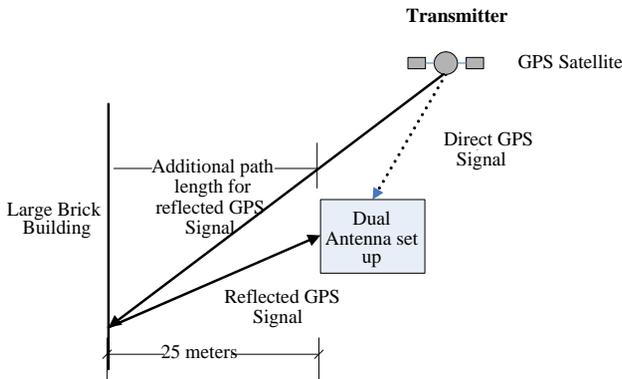
**Figure 7.** Set up for detection of reflected GPS signals.
