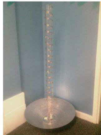
Figure 6. Assembled LHCP helical antenna.
