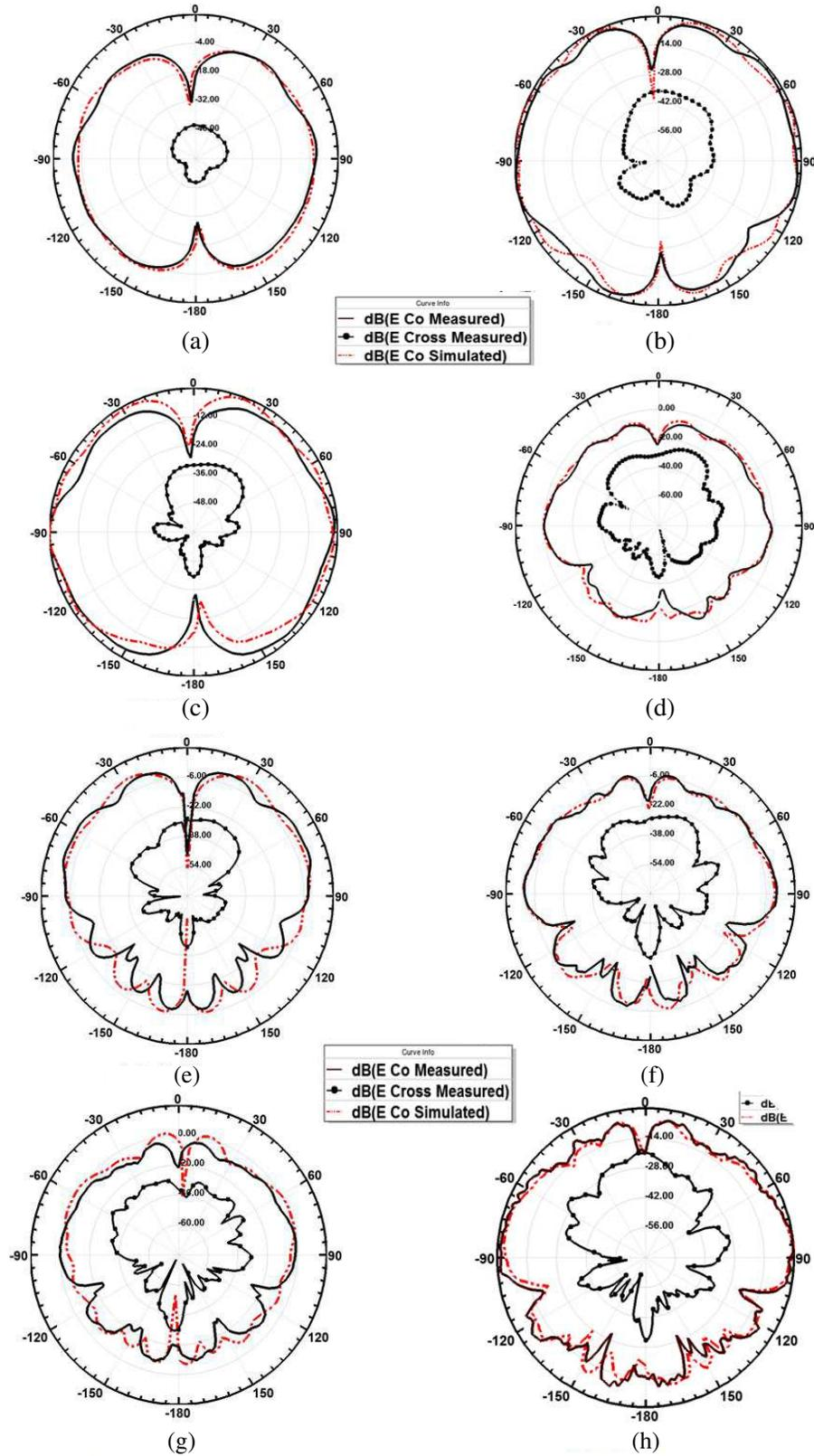
**Figure 12.** Antenna  $E$  plane measured and simulated radiation patterns in  $yz$  plane. (a) At 2 GHz. (b) At 4 GHz. (c) At 6 GHz. (d) At 8 GHz. (e) At 10 GHz. (f) At 12 GHz. (g) At 15 GHz. (h) At 18 GHz.
