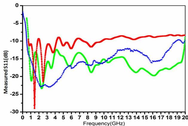
**Figure 13.** Red curve represents the antenna's simulated result with modified single planar vertical strip monocone antenna. Green curve represents the simulated result with modified double planar vertical strip monocone antenna, and blue curve represents the measured result for the modified double planar vertical strip monocone antenna.
