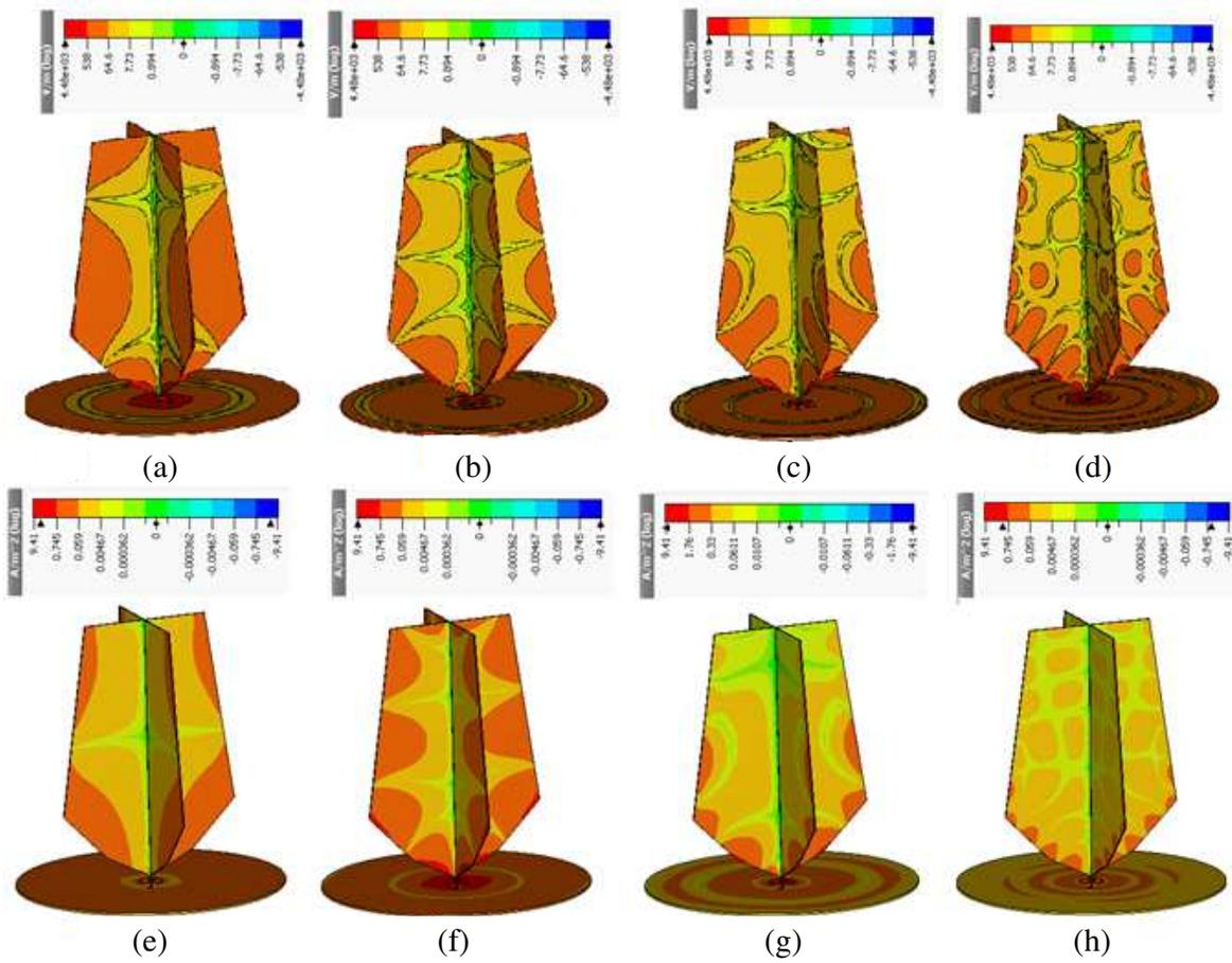
**Figure 8.** Simulated Current density and  $E$  field plots. (a) Current density @ 4 GHz. (b) Current density @ 8 GHz. (c) Current density @ 12 GHz. (d) Current density @ 16 GHz. (e) Electric field @ 4. (f) Electric field @ 4. (g)  $E$  field @ 12 GHz. (h)  $E$  field @ 16.
