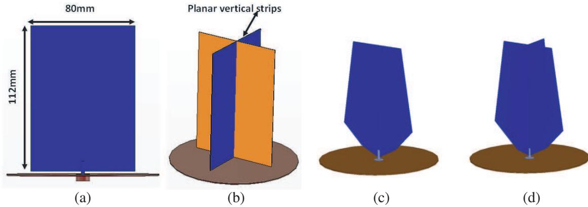
**Figure 3.** Simulated antenna (using HFSS) model phase 1 is shown in section (a), (b) and simulated antenna model phase 2 is shown in section (c), (d). (a) Antenna with single rectangular vertical strip. (b) Antenna with double rectangular vertical cross strips. (c) Antenna with modified single planar vertical strip. (d) Antenna with modified single planar cross vertical strip.
