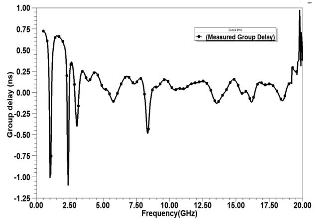
Figure 15. Measured group delay of fabricated antenna.
