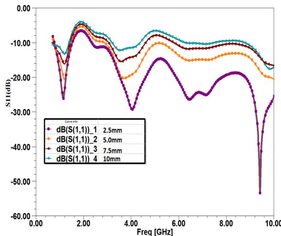
**Figure 11.**  $S$  parameter plot for parametric analysis of feed gap distance of double planar vertical strip antenna. (Using CST).
