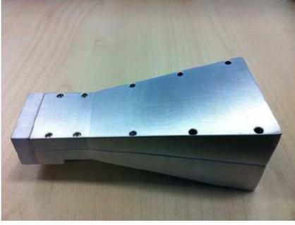
**Figure 8.** Prototype of the feed pyramidal horn antenna.
