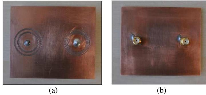
**Figure 9.** (a) Front and (b) back view of fabricated prototype of proposed power plane with MCSRs etched on it.
