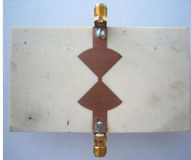
**Figure 2.** Photograph of the prototype of the proposed one-to-two bandpassing power divider.
