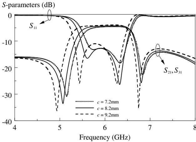
**Figure 11.** Effect of the arc-shaped slot length  $c$  on the frequency response of the one-to-two power divider.
