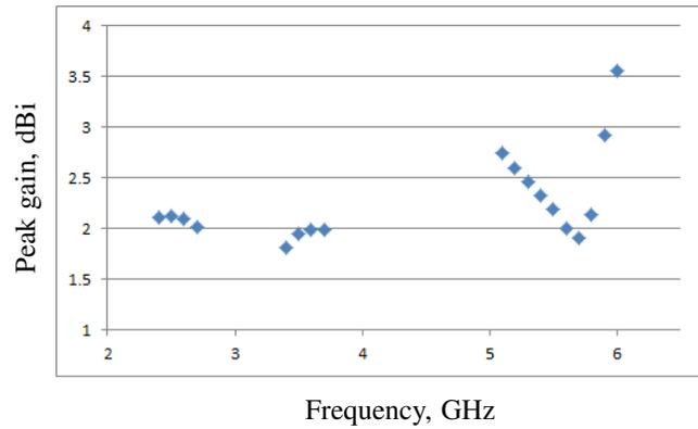
**Figure 8.** Peak gain of the proposed antenna.
