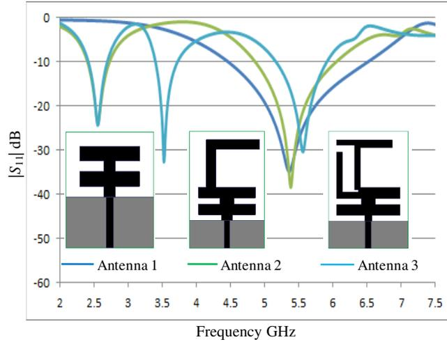
**Figure 2.** Simulated frequency responses of single-/dual-/tri-band antennas.
