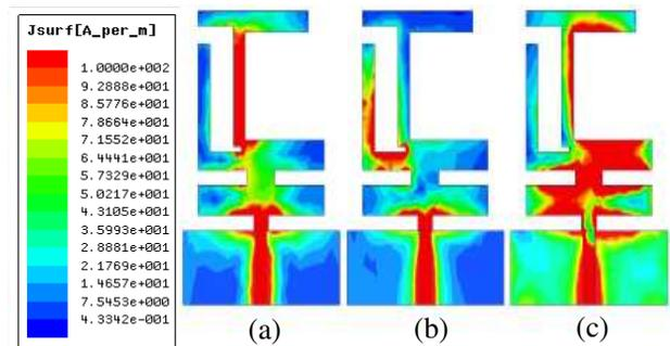
Figure 6. Simulated surface current distribution of the tri-band antenna at (a) 2.5 GHz, (b) 3.5 GHz, and (c) 5.5 GHz.
