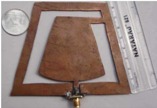
Figure 15. Photograph of fabricated SPICMA.
