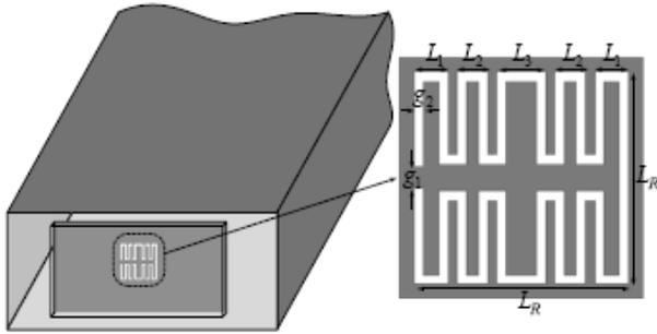
**Figure 1.** Simulative demonstration and geometry of the compact CSRR.
