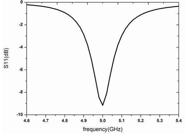
**Figure 2.** Simulated  $S_{11}$  of compact CSRR in a rectangular waveguide.
