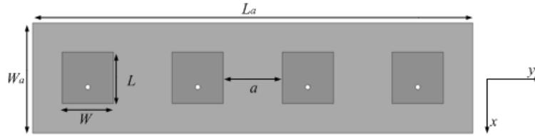
Figure 5.  $1 \times 4$  patch antenna array.
