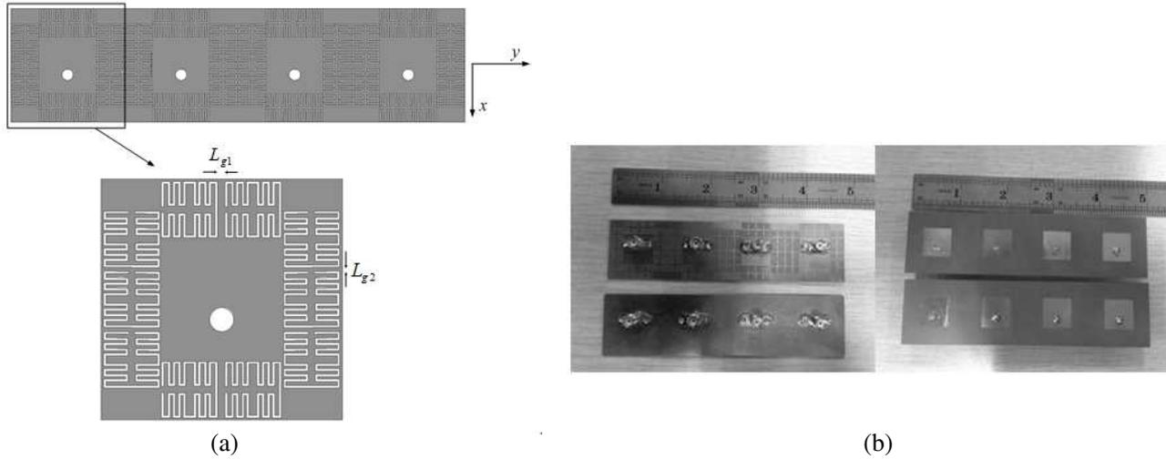
Figure 6. (a) Geometry of the patch antenna array with CSRRs etched on the ground. (b) Photograph of the patch array antennas with and without CSRRs.
