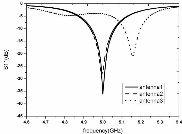
Figure 4. Simulated  $S_{11}$  of the microstrip antennas.
