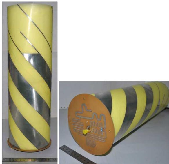
**Figure 5.** Fabricated antenna model.
