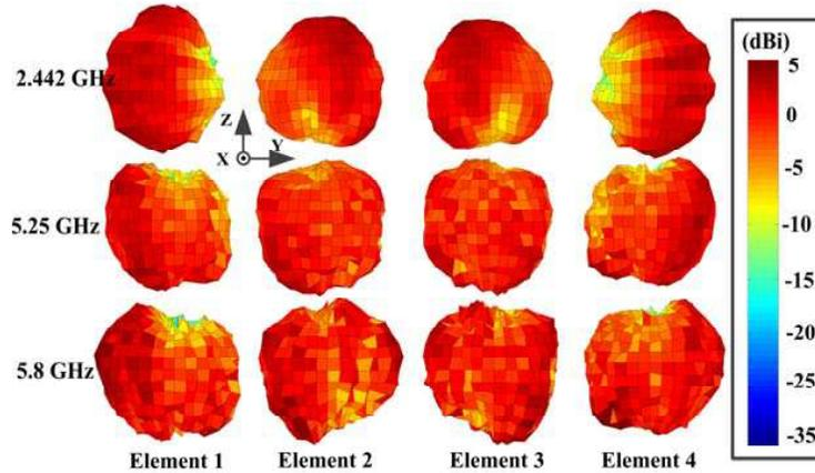
Figure 11. Measured 3-D radiation patterns at 2.442, 5.25, and 5.8 GHz.
