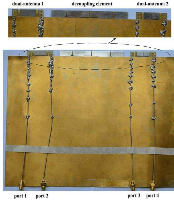
**Figure 9.** Photo of the fabricated quad-antenna system.
