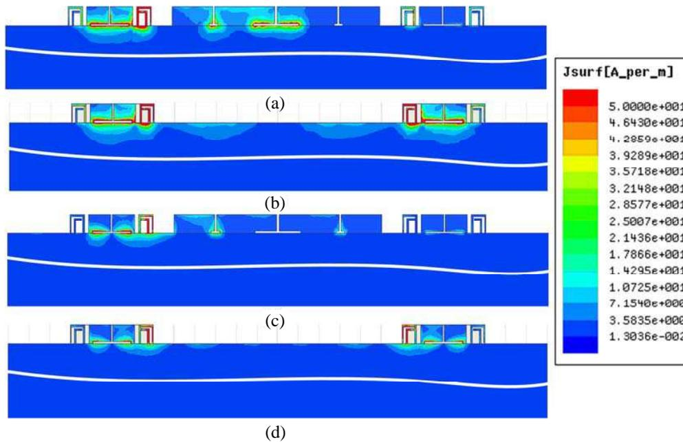
**Figure 5.** Simulated surface current distributions on the proposed antenna with and without the decoupling element at 2.442 GHz and 5.5 GHz. (a) With the decoupling element at 2.442 GHz. (b) Without the decoupling element at 2.442 GHz. (c) With the decoupling element at 5.5 GHz. (d) Without the decoupling element at 5.5 GHz.
