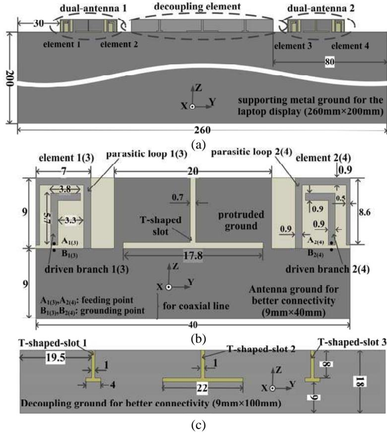
**Figure 1.** Geometry of the proposed quad-antenna system with dimensions in millimeters. (a) Installation positions of the two dual-antenna system and the decoupling element with their grounds connecting to the supporting ground. (b) Detailed dimensions of the dual-antenna system and its ground on the PCB. (c) Detailed dimensions of the decoupling element and its ground on the PCB.
