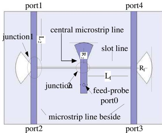
**Figure 2.** Structure of the feed network.
