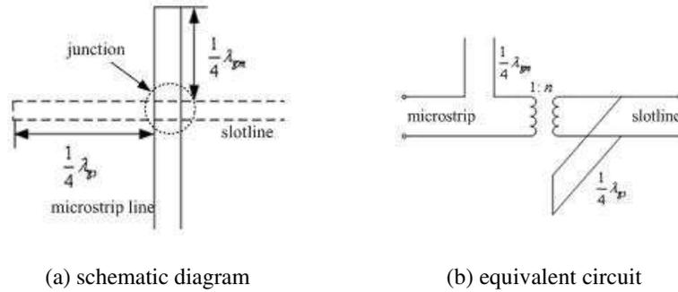
**Figure 1.** The microstrip/slotline transition.
