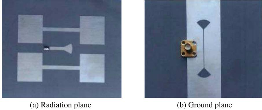
Figure 6. Photograph of fabricated antenna.
