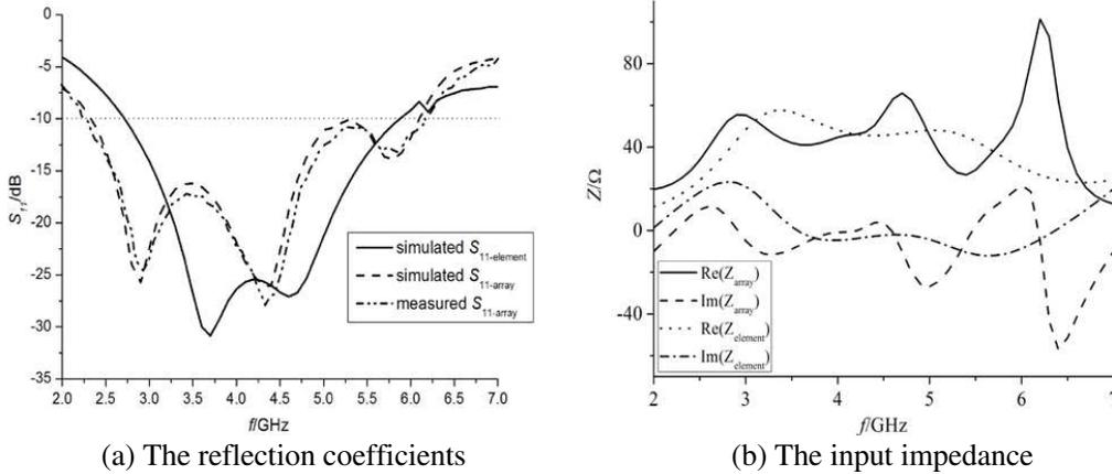
Figure 7. The reflection coefficients and input impedance of the antenna array and element.
