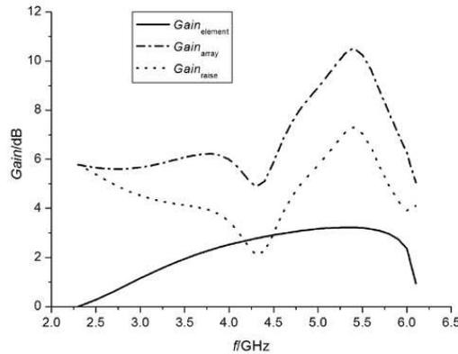
Figure 8. The gain of the UWB array and the element.
