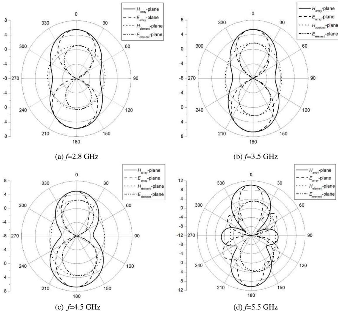
Figure 9. The radiation pattern of the array and the element.
