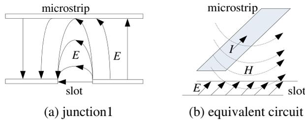
Figure 4. The electromagnetic field distribution in the sections of junctions.
