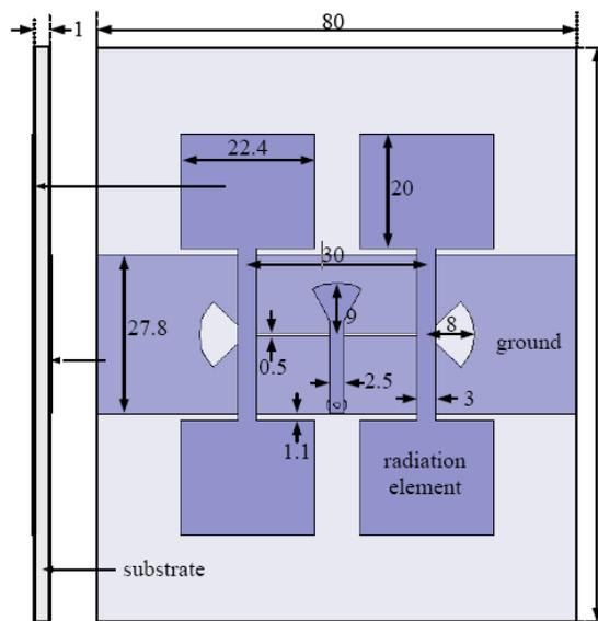
Figure 5. Structure of the antenna array (Units: mm).
