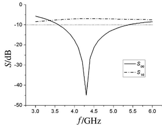
**Figure 3.** The reflection and transmission coefficient of the network.
