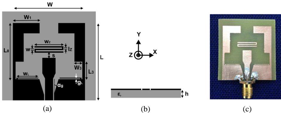
**Figure 1.** Geometry of the proposed dual band-notched UWB antenna, (a) top view, (b) side view, (c) fabricated antenna.  $L \times W \times h = 30 \text{ mm} \times 27 \text{ mm} \times 1.6 \text{ mm}$ ,  $L_0 = 21.8 \text{ mm}$ ,  $W_1 = 10 \text{ mm}$ ,  $L_3 = 6.8 \text{ mm}$ ,  $W_3 = 3 \text{ mm}$ ,  $\alpha_g = 16.7^\circ$ ,  $w_z = 10.8 \text{ mm}$ ,  $l_z = 0.5 \text{ mm}$ ,  $s = 2 \text{ mm}$ ,  $w = 0.5 \text{ mm}$ ,  $w_L = 8.2 \text{ mm}$ ,  $g_L = 0.3 \text{ mm}$ .
