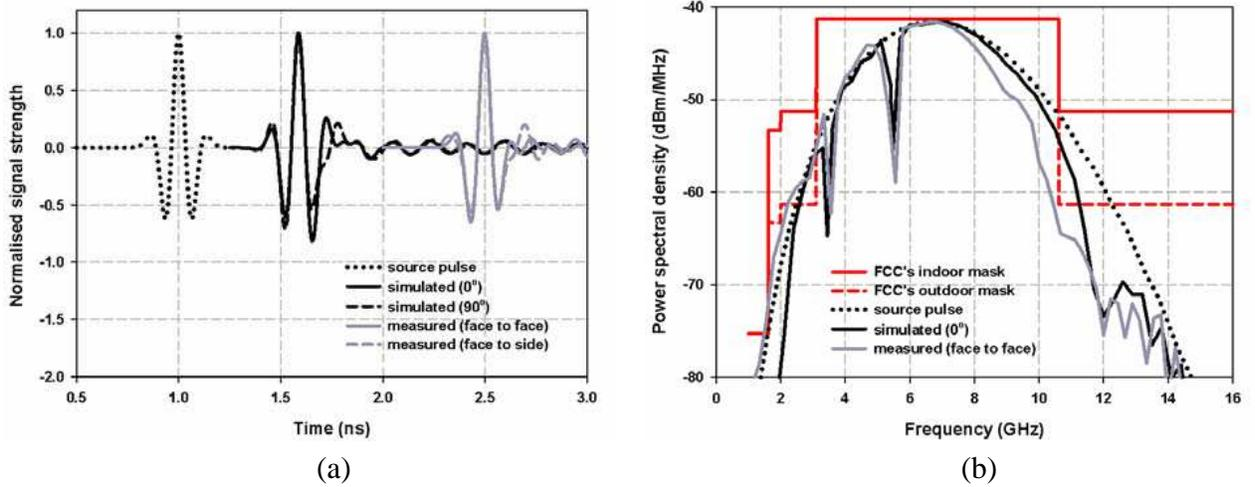
**Figure 12.** (a) Measured and simulated normalised radiated pulses for two different orientations. (b) Spectrum of source pulse and radiated pulses normalised to the FCC’s indoor and outdoor emission masks.
