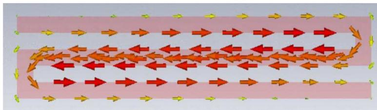
Figure 4. Simulated surface current distribution on Z-shaped parasitic element at 3.4 GHz.
