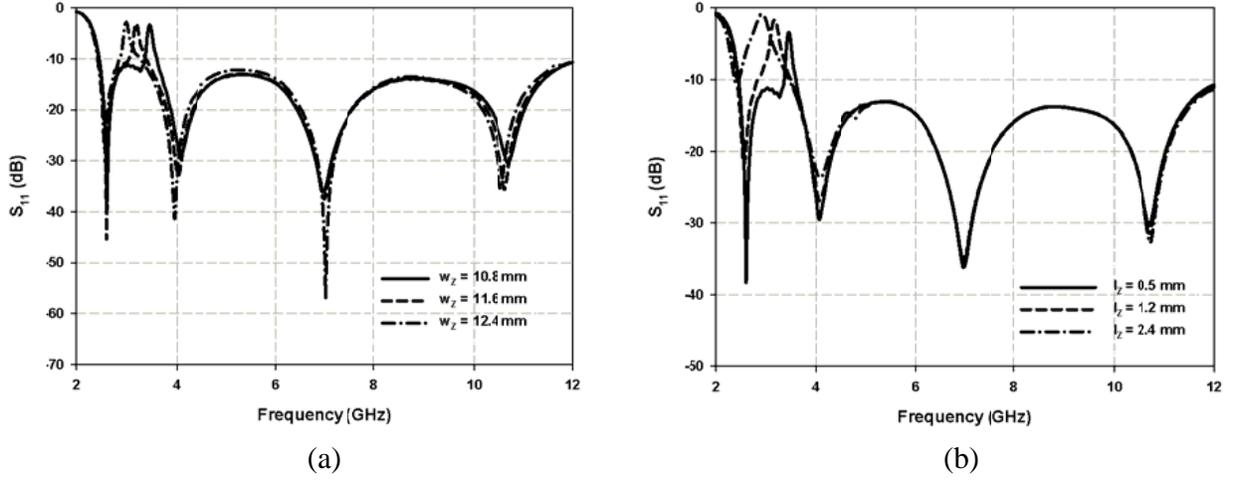
**Figure 5.** Effects of (a) horizontal strip length  $w_z$  and (b) vertical strip length  $l_z$  of Z-shaped parasitic on reflection coefficient of the single band-notched UWB antenna with all the other parameters same as in Figure 1.
