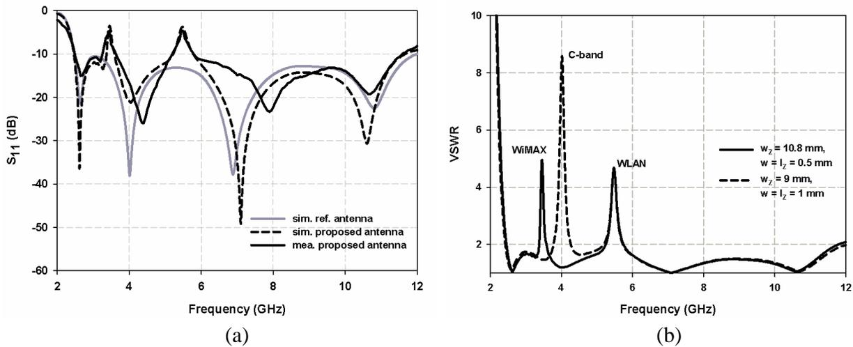
**Figure 8.** (a) Measured and simulated reflection coefficient of the proposed antenna. (b) Simulated VSWR of the proposed antenna with WiMAX/WLAN and C-band/WLAN notched bands (all the other parameters same as in Figure 1).
