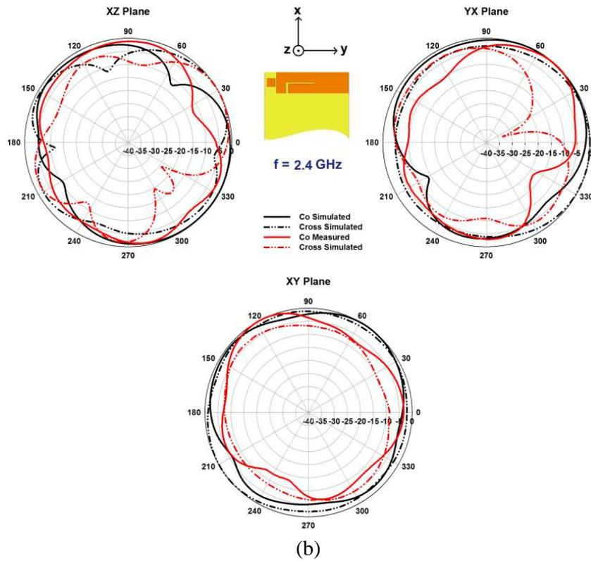
**Figure 8.** (a) Radiation patterns at 1.5 GHz for the proposed PIFA. (b) Radiation patterns at 2.4 GHz for the proposed PIFA.
