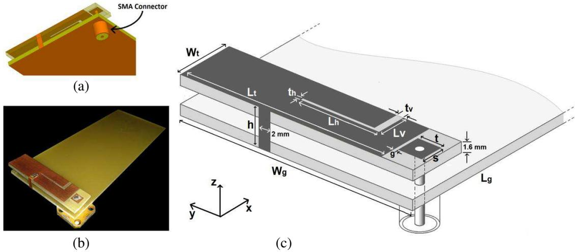
**Figure 1.** (a) HFSS layout, (b) fabricated PIFA, (c) geometry of the proposed PIFA. The optimised design parameters are  $W_t = 10$  mm,  $L_t = 34.5$  mm,  $L_h = 13.5$  mm,  $L_v = 5$  mm,  $h = 6$  mm,  $W_g = 40$  mm,  $L_g = 100$  mm,  $t_h = 0.5$  mm,  $t_v = 1.2$  mm,  $g = 0.5$  mm,  $s = 4$  mm and  $t = 4$  mm.
