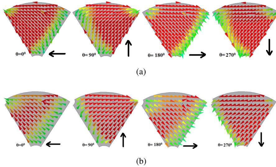
**Figure 4.** Simulated current distribution on the patch at four different phase angles in (a) Antenna 1 at 1990 MHz; (b) Antenna 2 at 2005 MHz.
