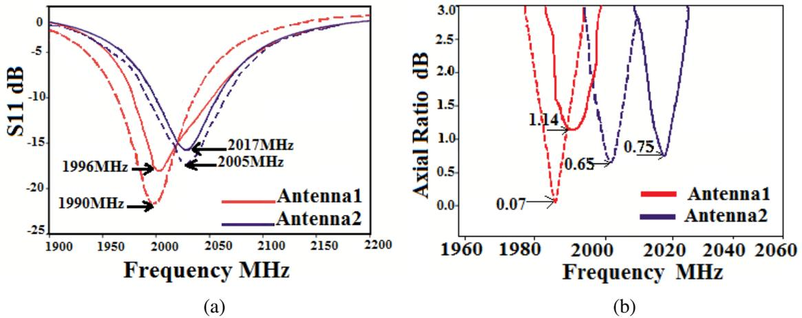
Figure 3. Simulated (dotted line) and measured (solid line) characteristics of Antenna 1 & Antenna 2 with  $r = 6.6$  mm,  $r_1 = 3$  mm. (a)  $S_{11}$  (10 dB return loss). (b) Axial ratio.
