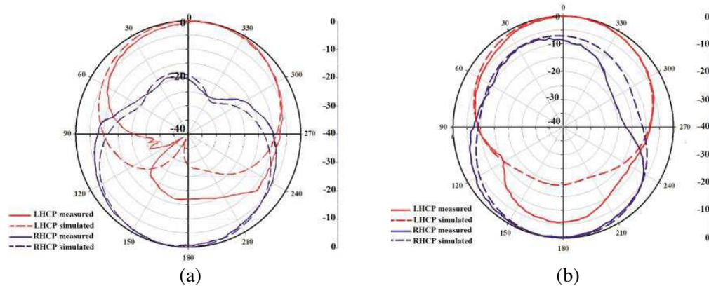
**Figure 7.** Simulated and measured radiation patterns in two orthogonal planes for Antenna 1 at  $f_c = 1996$  MHz. (a)  $YZ$  plane. (b)  $XZ$  plane.
