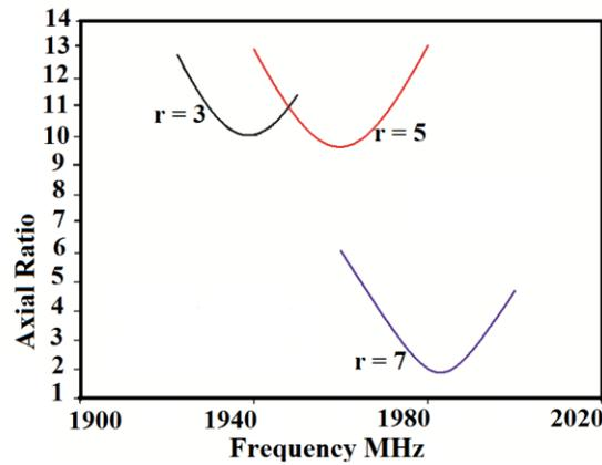
Figure 2. Simulated axial ratio characteristics of Antenna 1 for variation of the parameter  $r$ .
