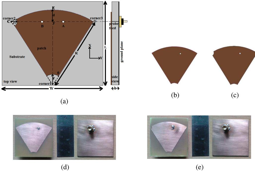
**Figure 1.** Geometry of the proposed antennas. (a) Top view and side view of the proposed antenna structure. (b) Top view of the fan-shaped patch in Antenna 1. (c) Top view of the patch in Antenna 2. (d) Photograph of Antenna 1. (e) Photograph of Antenna 2.
