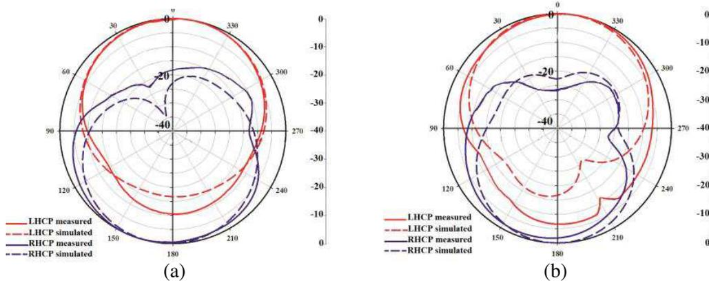
**Figure 8.** Simulated and measured radiation patterns in two orthogonal planes for Antenna 2 at  $f_c = 2017$  MHz.
