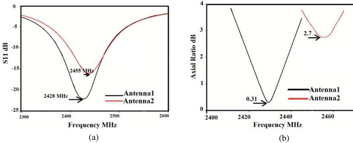
**Figure 6.** Simulated characteristics at frequency 2.4 GHz. (a) Return loss. (b) Axial ratio.
