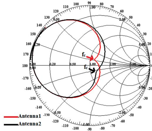
**Figure 5.** Smith chart of Antenna 1 and Antenna 2 (Simulated).
