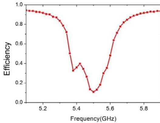
**Figure 10.** Simulated efficiency of the proposed antenna.
