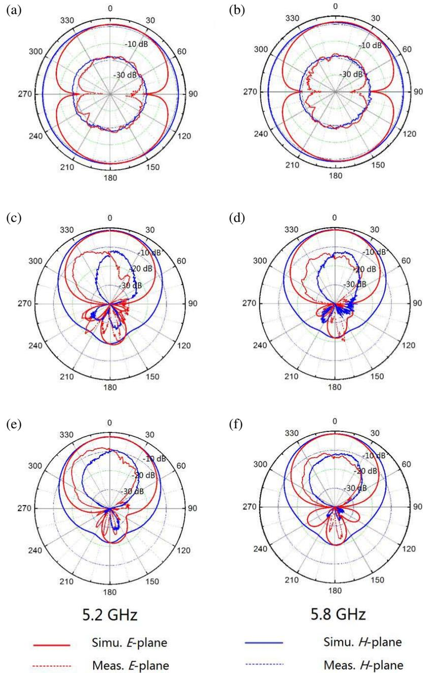
**Figure 7.** Simulated and measured *E*-plane and *H*-plane radiation pattern of (a), (b) the monopole, (c), (d) integrated PEC-enabled antenna and (e), (f) the metasurface-enabled antenna at two different resonant frequencies.
