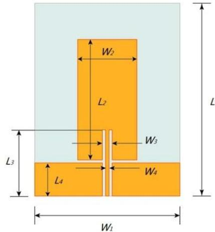
**Figure 1.** Top view of the monopole.
