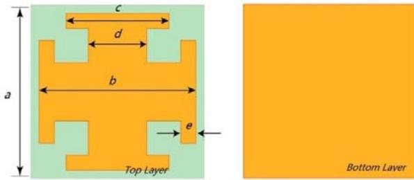
**Figure 2.** Geometry and dimensions of the JC based metasurface.
