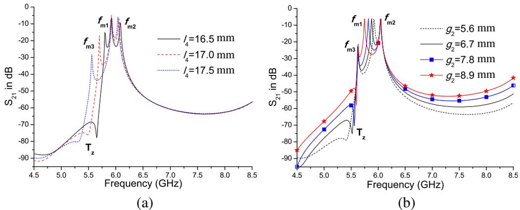
**Figure 2.** The insertion losses of the filter with varied  $l_4$  and  $g_2$  in the weak coupling case: (a) varied  $l_4$  with fixed  $g_2 = 5.6$  mm, (b) varied  $g_2$  with fixed  $l_4 = 17.25$  mm.
