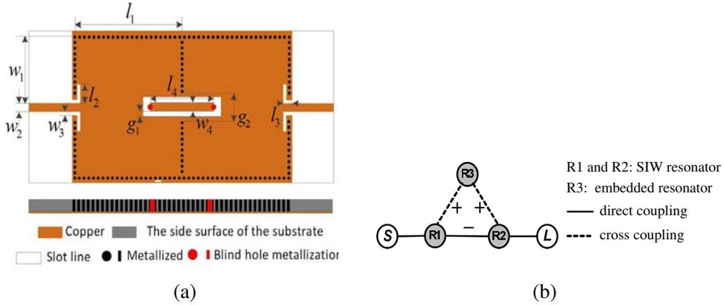
**Figure 1.** (a) Schematic, and (b) coupling scheme of the inline triplet SIW bandpass filter. ( $l_1 = 22.8$  mm,  $l_2 = 3.5$  mm,  $l_3 = 1.3$  mm,  $l_4 = 17.25$  mm,  $g_1 = 0.25$  mm,  $g_2 = 5.6$  mm,  $w_1 = 12.5$  mm,  $w_2 = 1.588$  mm,  $w_3 = 0.3$  mm,  $w_4 = 1.5$  mm).
