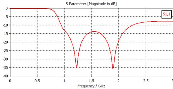
Figure 5. Return loss of the proposed antenna.
