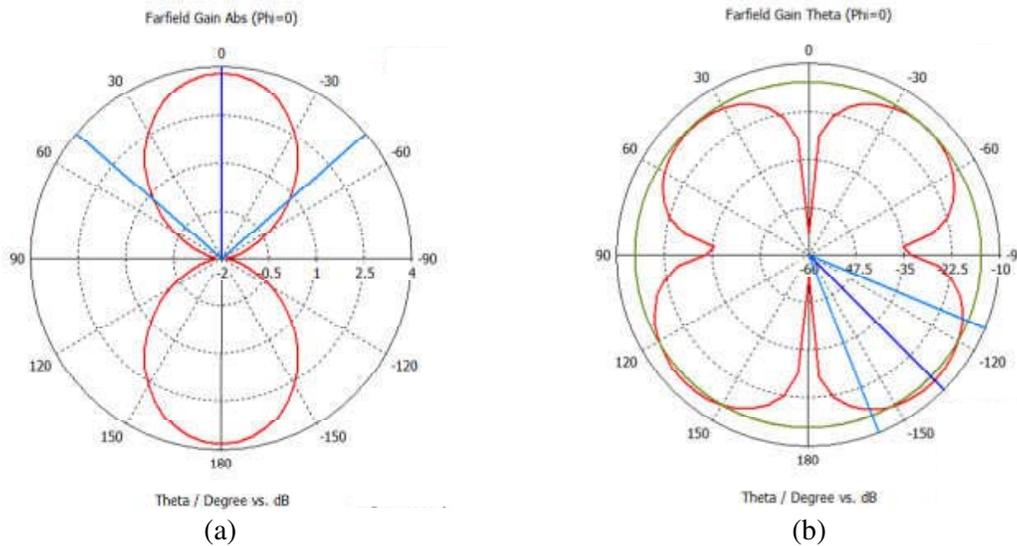
Figure 7. Radiation pattern of the proposed antenna (a) *E*-plane and (b) *H*-plane.
