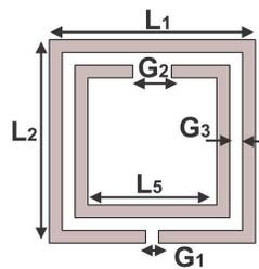
**Figure 2.** Square SRR structure with parameters.
