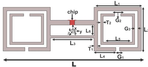
**Figure 1.** Schematic diagram of the proposed RFID tag.
