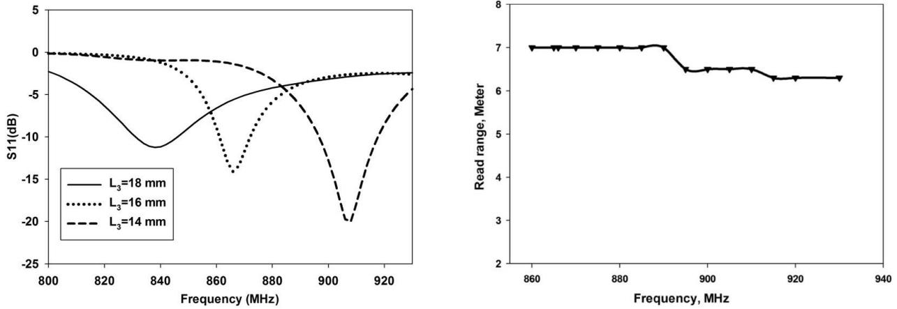
**Figure 8.** Simulated return loss of the proposed RFID tag antenna with parametric evaluation.
