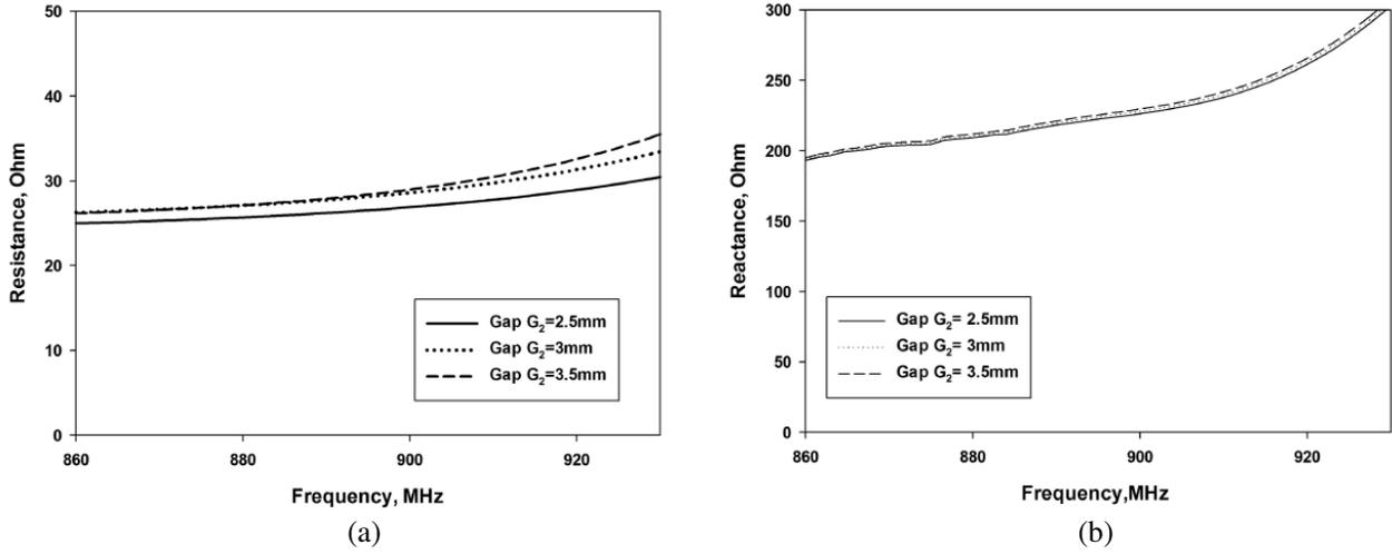
**Figure 7.** Variation of input impedance with frequency for different values of  $G_2$  ( $G_1 = 1.5\text{ mm}$ ). (a) Resistance Vs frequency. (b) Reactance Vs frequency.
