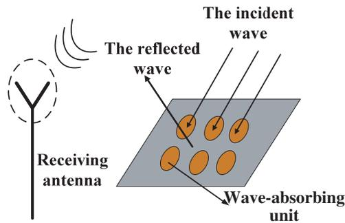
**Figure 1.** Equivalent wave-absorbing diagram of receiving antenna.
