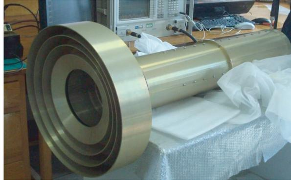
Figure 5. OMT prototype connected with a corrugated horn for measurement.
