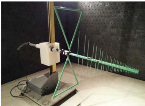
**Figure 5.** Monopole biconical antenna.
