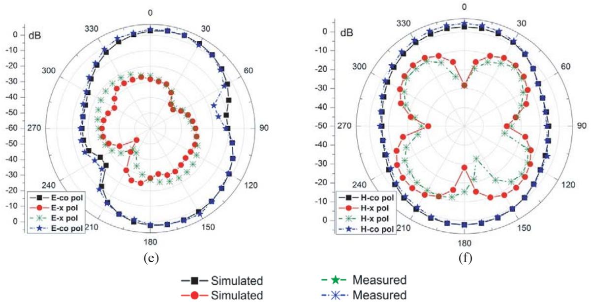
**Figure 13.** Simulated and measured  $E$ -field ( $XZ$  plane) and  $H$ -field ( $YZ$  plane). (a) 3.75 GHz ( $E$ -field), (b) 3.75 GHz ( $H$ -field), (c) 4.5 GHz ( $E$ -field), (d) 4.5 GHz ( $H$ -field), (e) 7.5 GHz ( $E$ -field), (f) 7.5 GHz ( $H$ -field).
