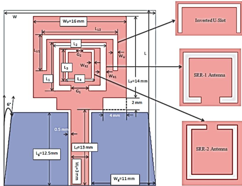
**Figure 1.** Proposed triple band notched UWB antenna integrated with inverted U-slot antenna, SRR-1 antenna and SRR-2 antenna.  $W = 26$  mm,  $L = 30$  mm,  $L_{U1} = 6.1$  mm,  $L_{U2} = 13$  mm,  $L_1 = 8.3$  mm,  $L_2 = 9$  mm,  $G_1 = 3$  mm,  $W_{R1} = 1$  mm,  $W_U = 0.8$  mm,  $L_3 = 5.38$  mm,  $L_4 = 4$  mm,  $W_{R2} = 0.48$  mm and  $G_2 = 1$  mm.
