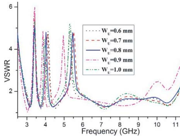
Figure 6. Inverted U slot width variation and VSWR.
