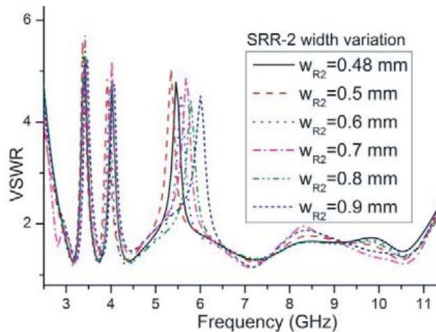
Figure 8. SRR-2 slot width and VSWR.
