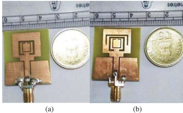
**Figure 2.** Proposed triple band stop antenna geometry. (a) Dual band notched UWB antenna. (b) Proposed band notched UWB antenna.
