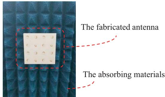
**Figure 8.** The fabricated antenna was measured in microwave darkroom.
