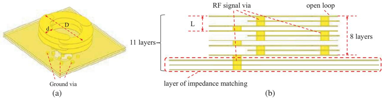
Figure 1. Structure of the proposed antenna element.
