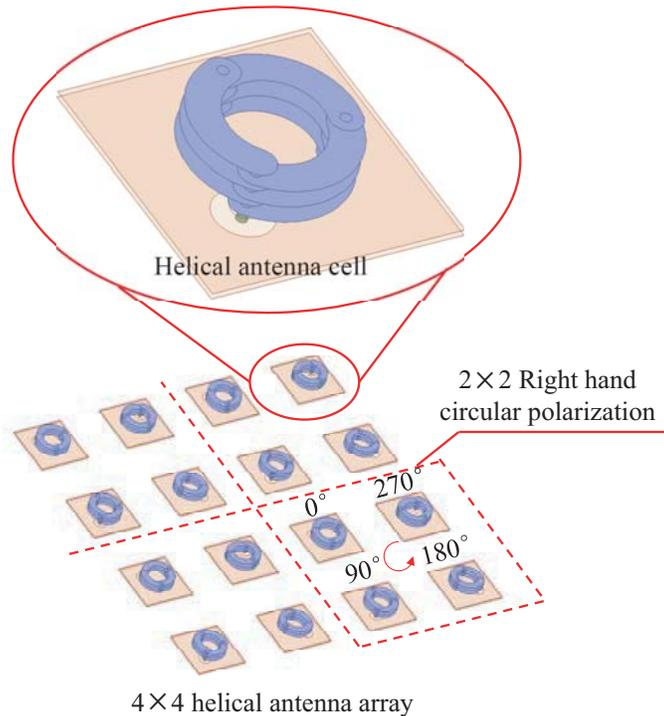
Figure 2. Structure of the proposed  $4 \times 4$  antenna array.
