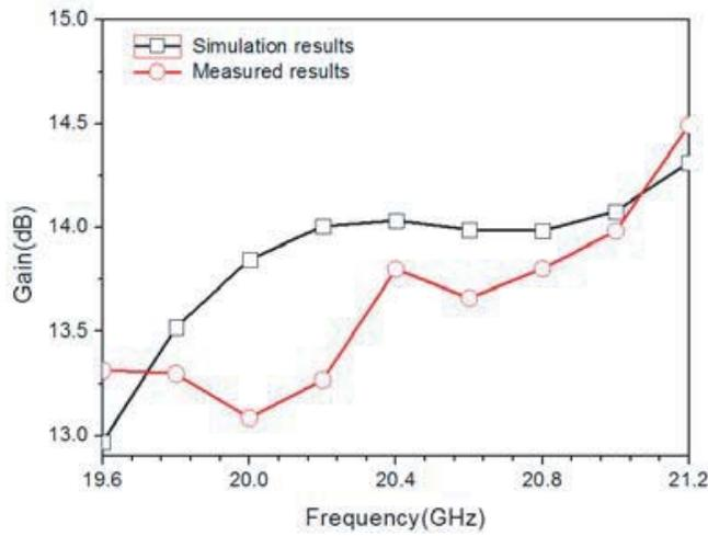
Figure 12. Gain performance of the proposed antenna array.
