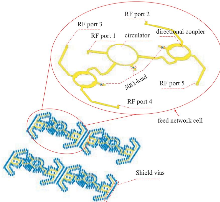
**Figure 4.** Structure of the proposed feeding network.
